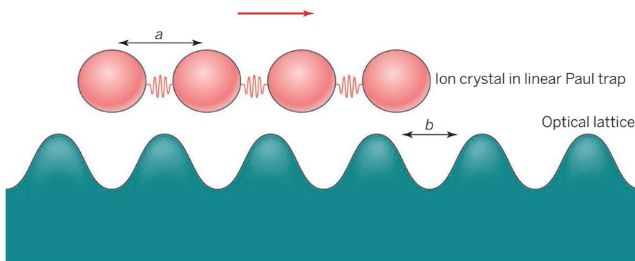
**The atomic friction simulator.** An ion crystal confined in a linear Paul trap is moved across a periodic optical lattice. Friction is found to depend strongly on the commensurability of these two lattices, even for systems with only two to six ions included in the trap.
