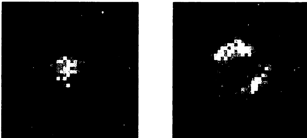
Figure 5-2: A round cloud pierced by a focused argon-ion laser beam in the magnetic trap. The round cloud of about 100 \mu\text{m} diameter was made by applying several tens of gauss magnetic bias field to the magnetic trap, weakening the radial confinement until it became comparable to the axial. An argon-ion laser beam was focused into the center of the cloud and repelled atoms due to the optical dipole force.
