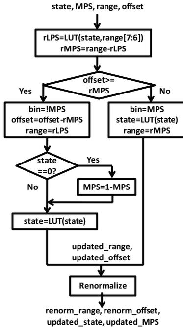
Fig. 1: Flowchart of binary arithmetic decoder in H.264/AVC CABAC [4].
