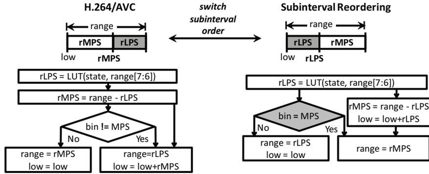
Fig. 3: Impact of subinterval reordering for CABAC encoding.
