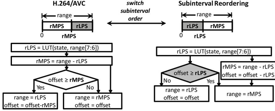
Fig. 2: Impact of subinterval reordering for CABAC decoding.
