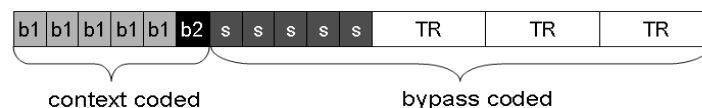
Figure 5: Parallel Context Processing (PCP) in coefficient levels. All bypass bins are grouped together to increase throughput.
