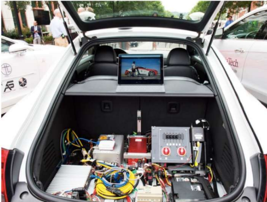
Shelley, a self-driving Audi TT developed by Stanford University, uses the brains in the trunk to speed around a racetrack autonomously.
