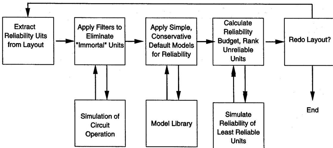
**Figure 1:** A flow chart for a full hierarchical circuit-level reliability assessment, the basis for the tool ERNI.
