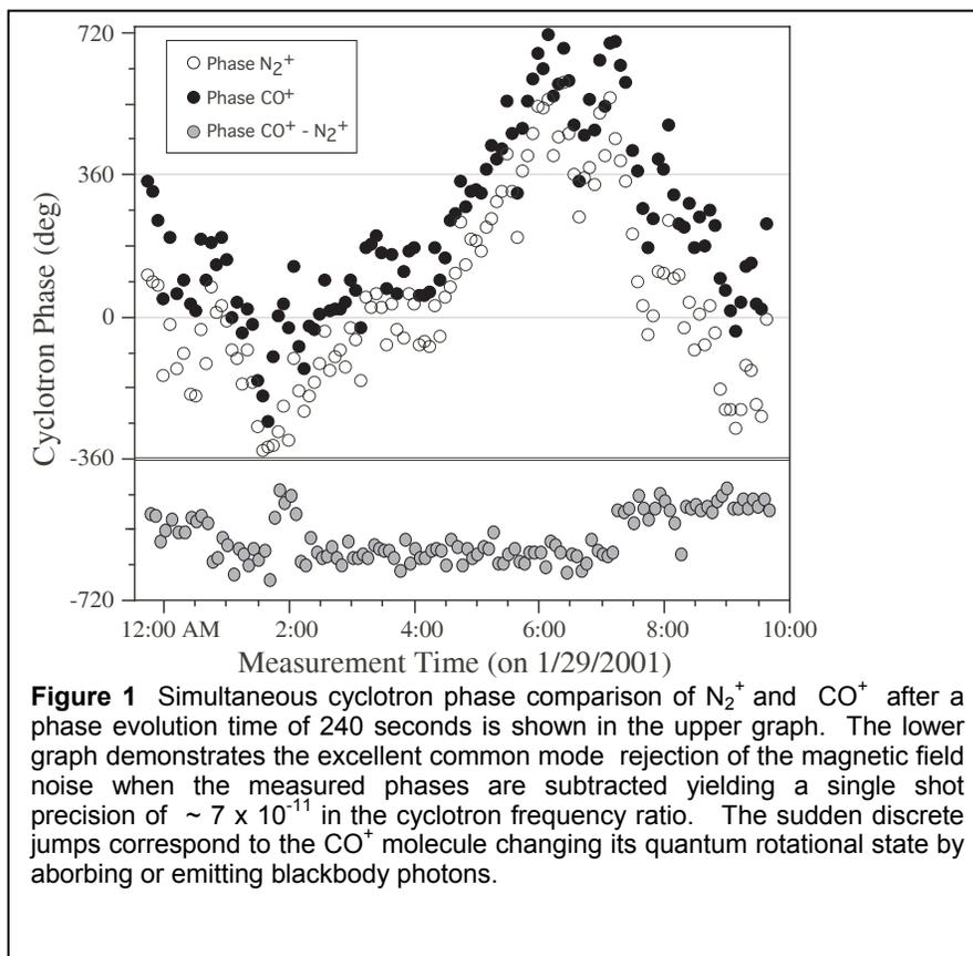
We have achieved averaging intervals lasting as long as 60 hours all under automated computer control and even during the daytime when magnetic field noise from the nearby subway prevents *alternate* ion comparisons with useful precision.
