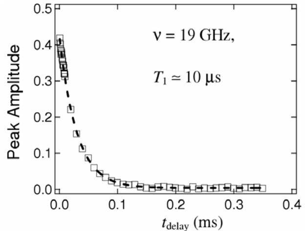
**Fig. 2.** Normalized resonant peak amplitude as a function of readout delay time  $t_{\text{delay}}$ . The dashed line is the best fit to exponential decay with a time constant  $T_1 = 10 \mu\text{s}$ . The experimental data show remarkable agreement with the theory prediction.
