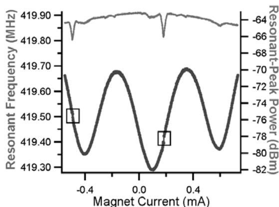
**Figure 2:** Experimental results at 300mK: the lower plot (left axis) shows the modulation of the resonant frequency with external magnetic field. Qubit steps corresponding to transitions between opposite flux states were observed at every 1.3 periods of the SQUID lobe. The upper plot (right axis) shows the corresponding peak amplitude of the resonant spectrum. The dip in peak power coincides with the qubit step.
