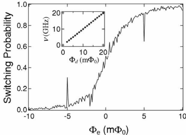
**Fig. 1.** Switching probability vs. external magnetic field with 10 GHz microwave irradiation. The resonant peak and the dip are caused by photon induced transition between two macroscopic quantum states. Inset: microwave frequency vs. the distance between the peak and the dip (symbols). The solid line is the theoretical calculation using qubit parameters.
