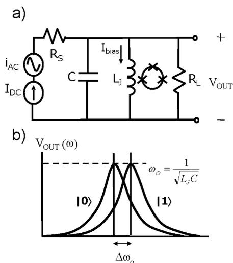
**Figure 1a:** The SQUID inductor is incorporated in a resonant readout circuit. It is inductively coupled to a PC qubit to detect its state. Figure 1b: A transition of the qubit state changes the Josephson inductance of the SQUID, and can be sensed as a shift in the resonant frequency of the readout circuit.
