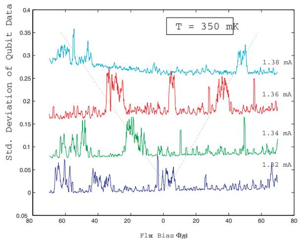
**Figure 2:** Data illustrating oscillator dependent excitations in the persistent-current qubit. As the current bias to the oscillator is increased the frequency of radiation produced by the oscillator also increases, and correspondingly, the excitations in the persistent-current qubit move away from one another, matching the quantized energy levels in the device.
