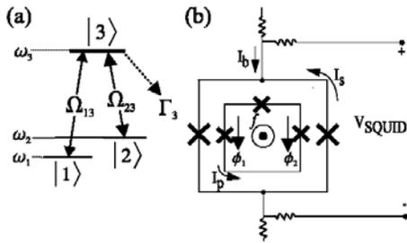
**Figure 1:** a. Energy level diagram of a three-level  $\Lambda$  system. EIT can occur in atoms possessing two long-lived states  $|1\rangle$ ,  $|2\rangle$ , each of which is coupled via resonant laser light fields to a radiatively decaying state  $|3\rangle$ . b. Circuit schematic of the persistent-current qubit and its readout SQUID.
