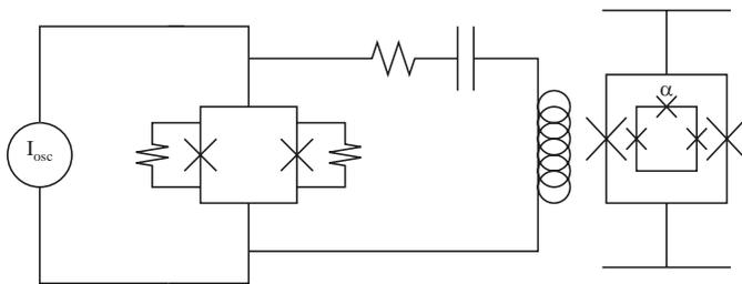
**Figure 1:** A schematic representation of the on-chip oscillator circuit with a bandpass filter, coupled inductively to the pc-qubit and measurement SQUID. When the oscillator is current biased above its superconducting critical current it emits radiation at a frequency that can be tuned by the current bias. The radiation can stimulate quantum transitions within the superconducting persistent-current qubit.
