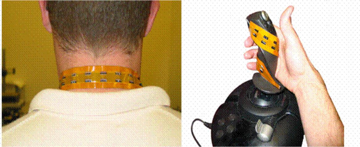
*Figure 4.3-1 Conformable tactile array based on shape memory alloy*
