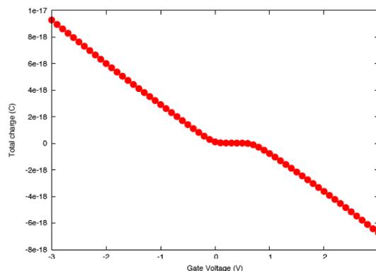
**Figure 2.** Total charge on nanotube surface versus gate voltage for a 50-nm dual-gate CNTFET. From this plot we estimate a total gate capacitance of 3.2 aF.
