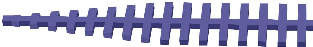
**Figure 1:** A taper transition from uniform waveguide to a slow light waveguide
