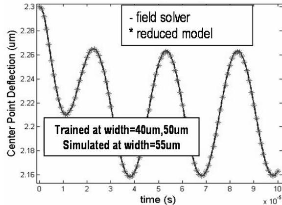
**Figure 2:** Center point deflection predicted by our parameterized reduced model of order 40, compared to a finite difference detailed simulation.
