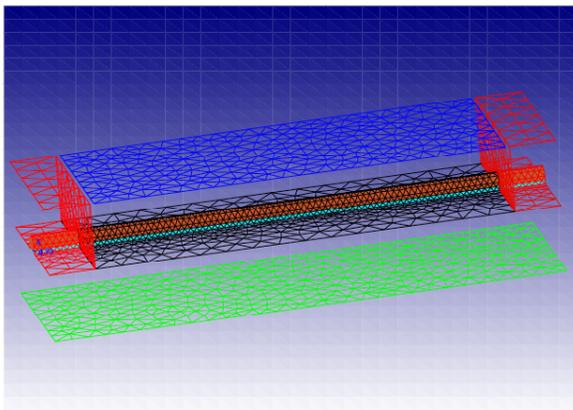
**Figure 1.** Discretized geometry of a 50-nm dualgate CNTFET. Green panels: bottom gate. Cyan panels: SiO<sub>2</sub>–air interface. Black panels: High-  $\kappa$  dielectric interface. Red panels: Source/Drain metallization. Blue panels: Top gate. Orange panels: Carbon nanotube. Note that our discretization accurately captures the immersion of the nanotube in the Pd source/drain contacts and in the high- $\kappa$  material in the channel region.
