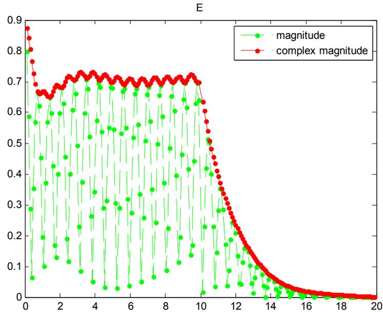
**Fig. 2:** The electrical field of a dielectric waveguide followed by an absorbing layer
