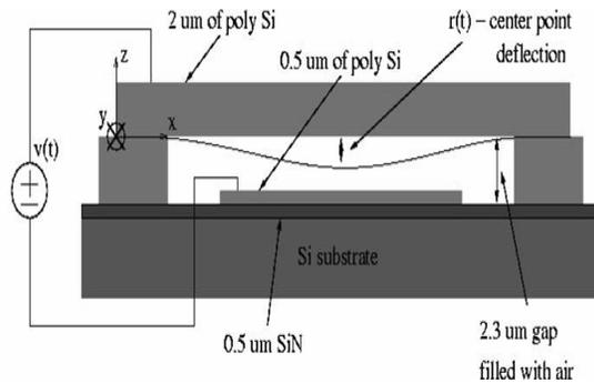
**Figure 1:** Application example: MEM switch realized by a polysilicon beam fixed at both ends and suspended over a semiconducting pad and substrate expansion.
