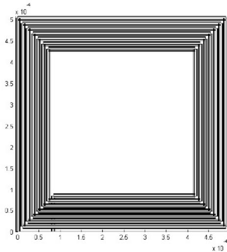
**Figure 1:** 7 turn RF inductor for which a parameterized (with respect to wire width and wire separation) reduced model has been constructed.
