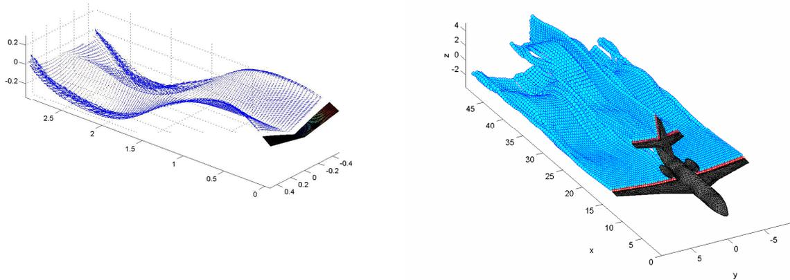
**Figure:** The above figures illustrate the combined boundary element method-vortex particle method approach for solving complex unsteady flows. The vortex particle representation of the lifting surface trailing vorticity is shown. The image on the left illustrates a flapping wing geometry, while the image on the right illustrates a rapidly heaving business jet.
