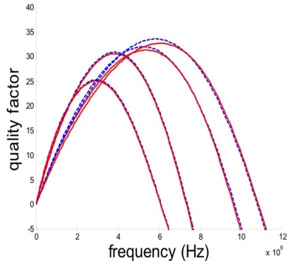
**Figure 2:** Matching of quality factor of 7 turn RF inductor when wire width = 16.5  $\mu\text{m}$ , wire separation = 1,5,18,20  $\mu\text{m}$ . Blue: Full model. Red: ROM.
