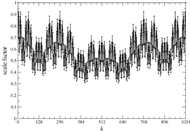
**figure 1.** The fractal rescaling factor for a sub-transform of size  $N=4096$  in order to achieve the new minimum-operation FFT.
