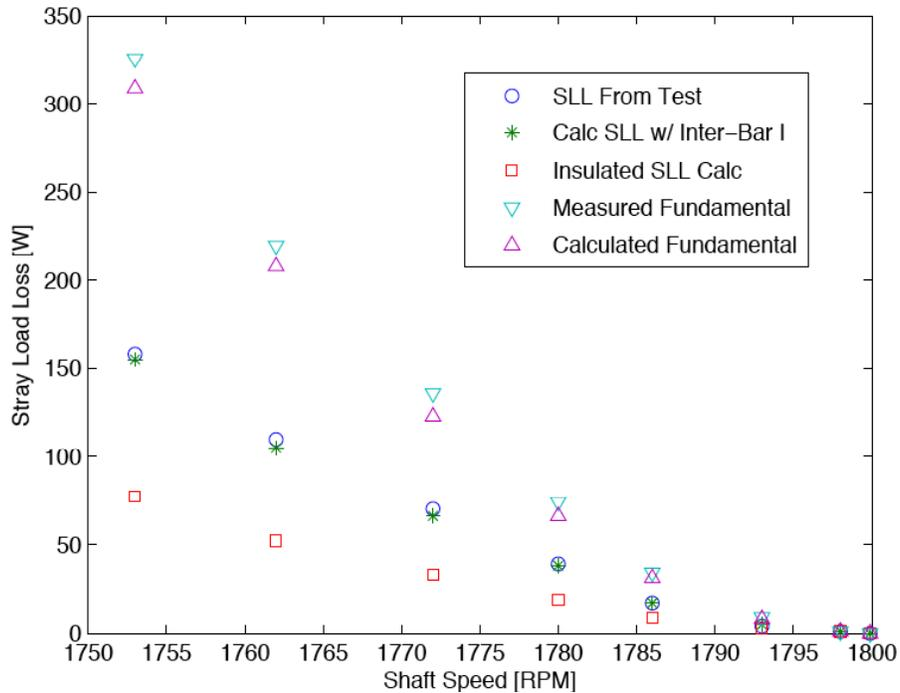
**Figure 6:** Comparison of measured and calculated fundamental and stray load loss for a 10 horsepower motor with a cast-copper rotor
