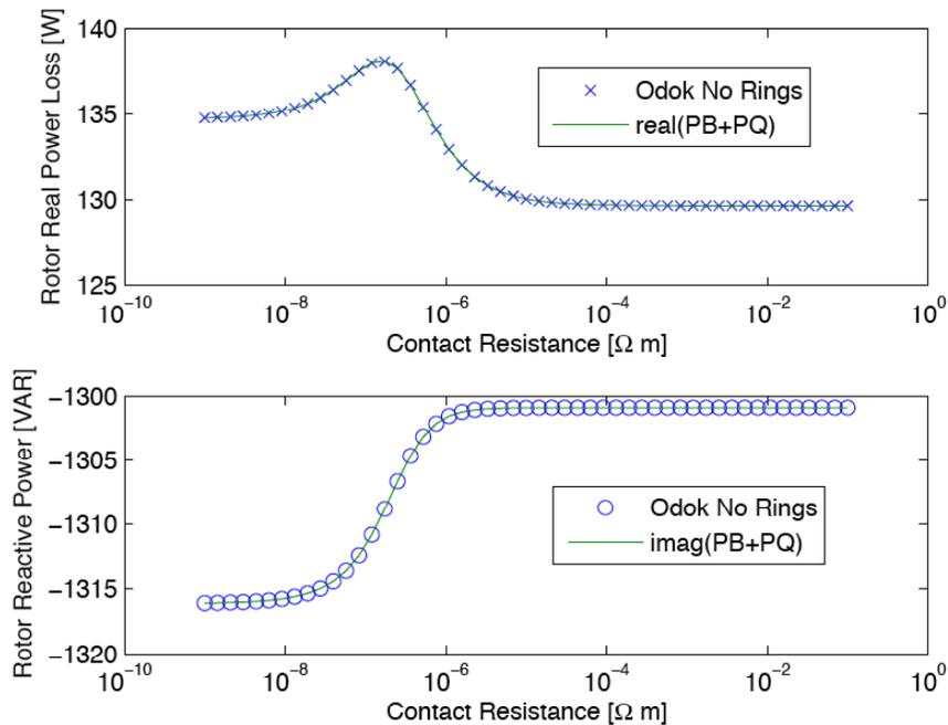
**Figure 5:** Odok's Calculation of rotor real and reactive loss for negligible end ring impedance.
