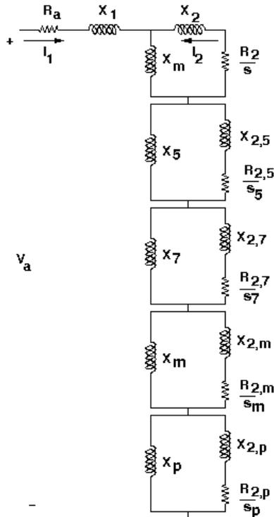
Figure 2: Extended Equivalent Circuit
