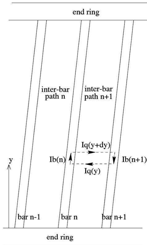
Figure 4: Illustration of skewed rotor bars<sup>5</sup>
