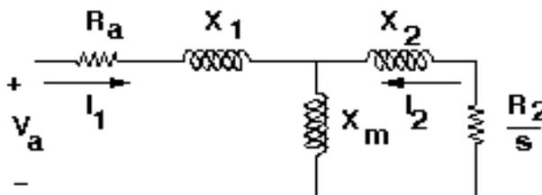
Figure 1: Induction Motor Elementary Circuit
