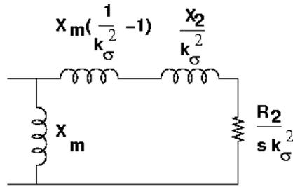
Figure 3: Rotor Section modified by Skew
