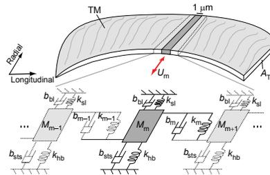
**Figure 7.** Incorporating effects of cochlear loads in the distributed impedance model of TM traveling waves.
