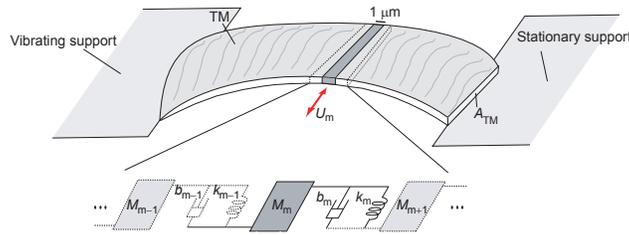
**Figure 4:** Model of TM wave motion. Longitudinal segments of the isolated TM are represented as discrete masses that are interconnected with springs that represent TM stiffness and dashpots that represent viscous loss in the TM.
