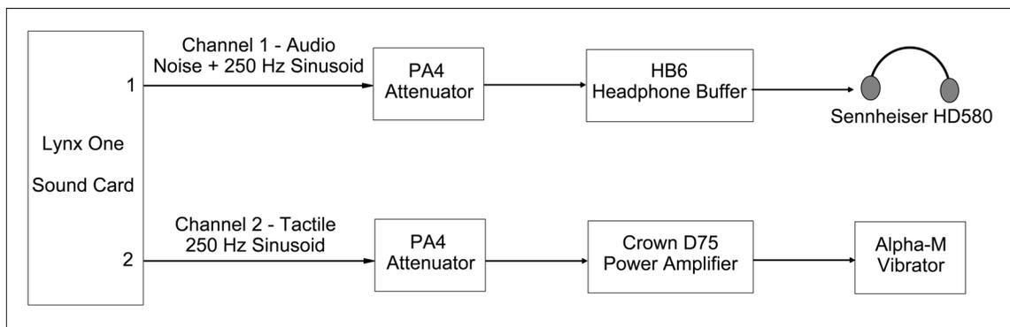
**FIG 1:** Block Diagram for Delivery of Auditory and Tactile Stimuli (demonstrating use of 250-Hz sinusoid in both modalities).
