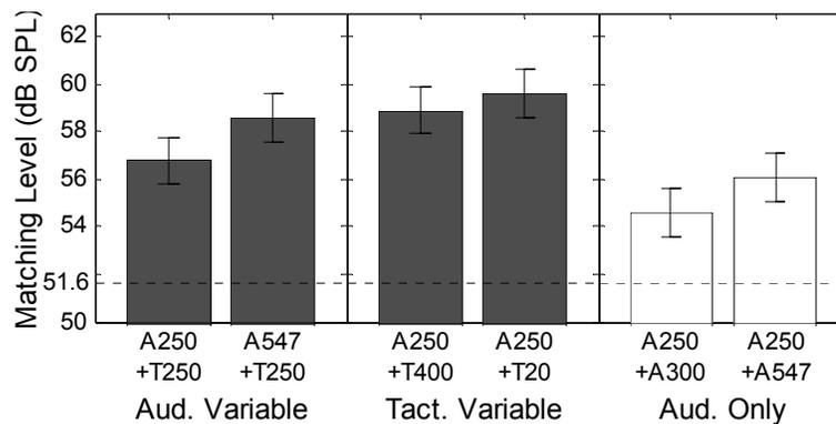
**FIG 2:** The average levels of the two-tone complexes when matched to the 25 dB SL 200-Hz tone. Error bars are one SEM.
