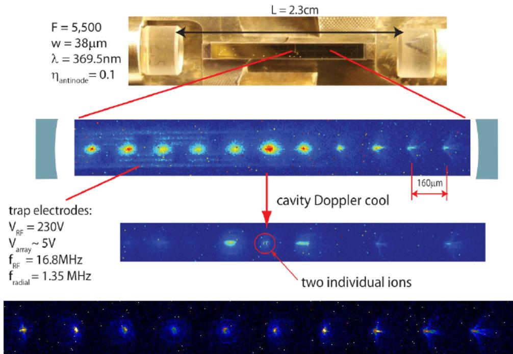
**Fig. 5. Microfabricated ion trap with optical resonator and image of ions trapped in array of Paul traps.** The top bar shows the microfabricated chip mounted inside a Fabry-Perot resonator of 2.3 cm length. The lower bars show pictures of trapped  $^{174}\text{Yb}^+$  ions excited by light circulating inside the optical resonator before and after Doppler cooling. The individual traps in the array are spaced by  $160\mu\text{m}$ , and located  $140\mu\text{m}$  above the chip surface.
