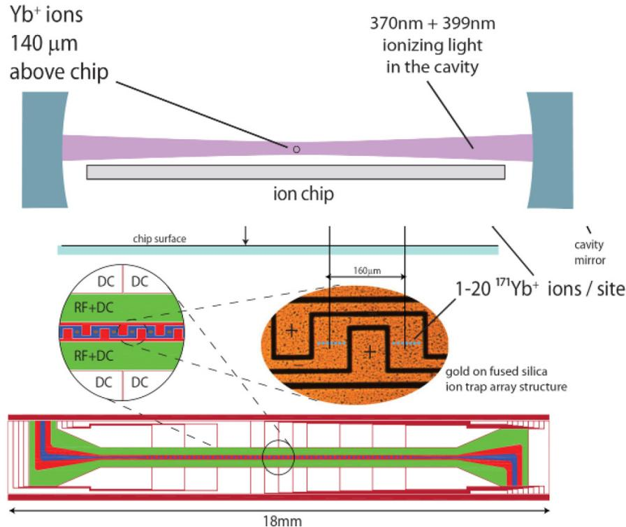
**Fig. 6. Details of the microfabricated ion trap.** The linear RF Paul trap is formed by three electrodes, where the outer two electrodes are driven at  $\sim 15$  MHz with respect to the middle electrode. The middle electrode is split into three parts to which different dc potentials can be applied (inset right), creating a periodic dc potential along the trap axis. A number of outer electrodes provide dc compensation along the trap.
