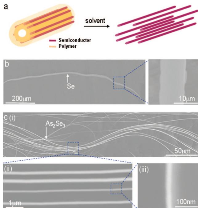
**Figure 4.** Semiconductor nanofilaments extracted from fiber. (a) The filament bundles are extracted from the fiber by dissolving the polymer matrix. (b) SEM micrograph of a Se filament and a magnified section of it. (c) (i) A bundle of  $\text{As}_2\text{Se}_3$  filaments. (ii) Magnified section showing parallel filaments. (iii) A section of a single filament.
