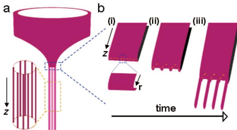
**Figure 5.** Proposed mechanism of filament arrays formation. (a) Schematic of a layer breakup into filaments during drawing. (b) (i–iii) A schematic of the time evolution of layer breakup. The formed viscous polymer/viscous glass interface has a cylindrical fluid front, whose breakup is driven by capillary instability.
