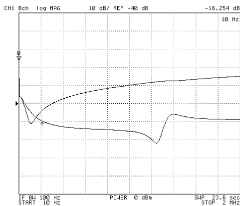
Fig. 15. Performance comparison between a 935C4W10K film capacitor and the inductance cancellation filter of Fig. 14.
