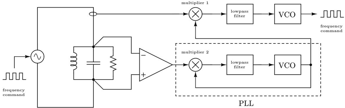
Fig. 3. Block diagram of a phase-lock tuning system.
