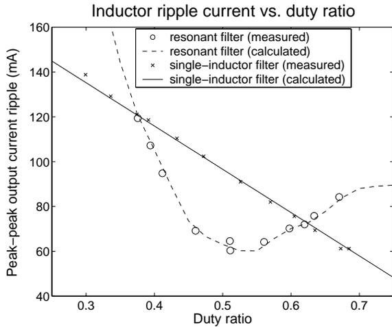
Fig. 8. Comparison of the peak-peak inductor ripple current performance of the single-inductor and resonant power stages.
