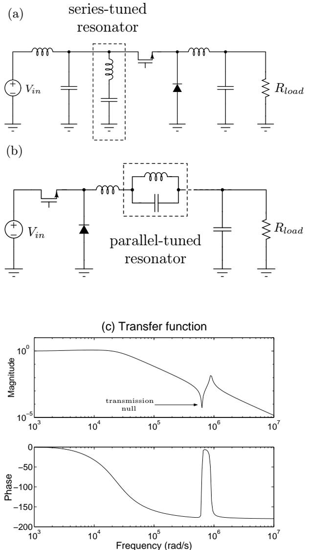
Fig. 2. Example of a series-resonant input filter for a buck converter. (a) The series-tuned leg provides a low-impedance current path (i.e. high attenuation) at a discrete frequency. (b) The parallel-tuned resonator presents a high impedance to switching ripple at a discrete frequency. (c) Transfer function: switch drain current to input current or switch source voltage to output voltage
