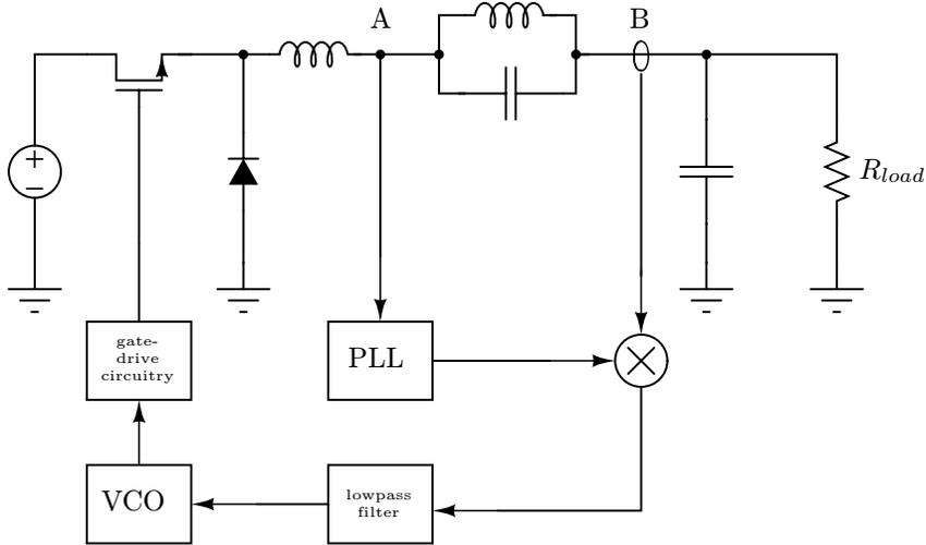
Fig. 5. Block diagram of phase-lock tuning system used to align a buck converter’s switching frequency to the maximum-impedance resonance of its output filter. A ground-referenced voltage measurement is made at point A, from which the AC voltage across the tank is determined. The resonator current is measured at point B.
