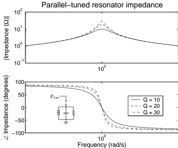
Fig. 1. Frequency response of second-order tuned circuits, normalized to the natural frequency  $\omega_n = 1/\sqrt{LC}$ . The impedance magnitude at a single frequency can indicate proximity to resonance (with calibration) but not whether resonance lies above or below the stimulus frequency. The impedance phase, however, increases or decreases monotonically, and its difference from  $0^\circ$  is an error signal indicating the distance and direction to resonance.
