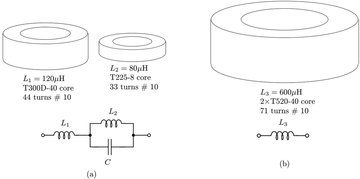
Fig. 6. Comparison of the core sizes for (a) resonant/low-pass and (b) simple low-pass magnetics for the power stage and input filter (primed values) of a 300W buck converter
