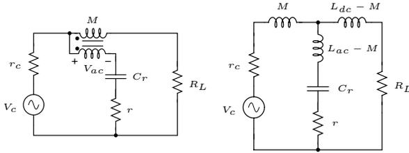
Fig. 12. Magnetically coupled shunt resonator and its equivalent T model, excited by a voltage source  $V_c$  representing the switch source node or output of a switching converter.
