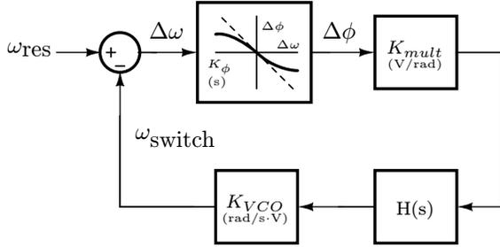
Fig. 11. Linearized tuning dynamics of the phase-sensing control system.
