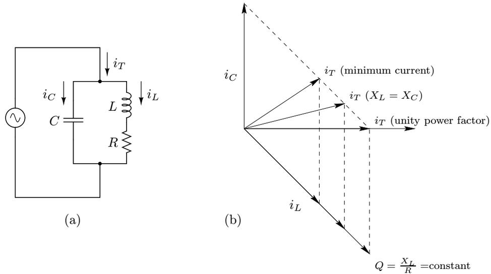
Fig. 4. Tuning points of a parallel-resonant circuit with low unloaded  $Q$ . **Note:** for inductor  $Q$  values above 10, these resonant points all converge to within 1% of frequency.
