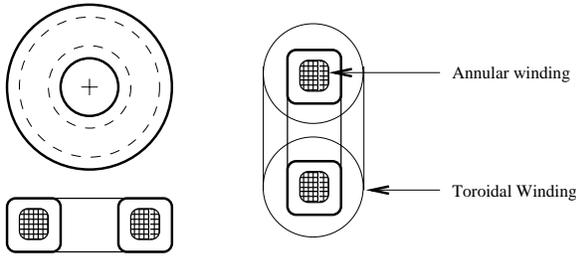
Fig. 13. Structural diagram of a cross-field reactor. The magnetic core is wound with two windings (an annular coil and a toroidal coil) that are not coupled in the usual sense.
