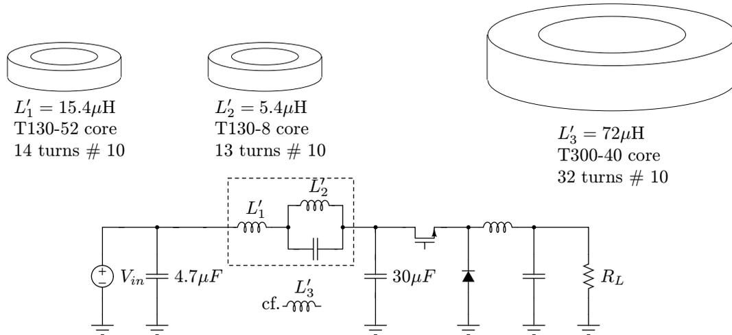
Fig. 7. Resonant input filter design for the prototype 300W buck converter
