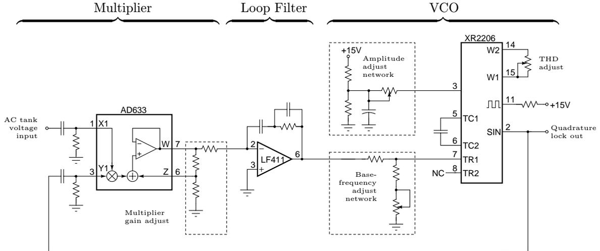
Fig. 10. Schematic of the PLL used in the prototype tuning system.
