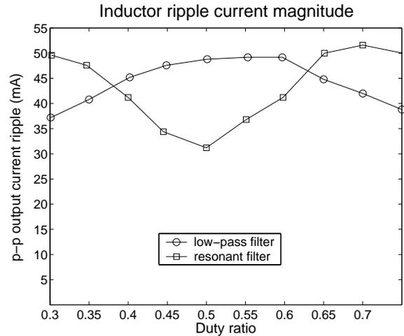
Fig. 9. Comparison of the peak-peak ripple performance of the single-inductor and resonant input filters.
