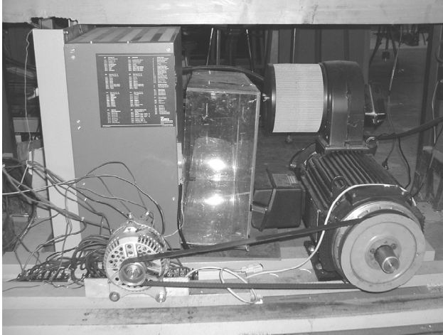
Fig. 13. The alternator and motor drive.
