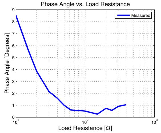
(b) Phase Angle of the Input Impedance vs. R
