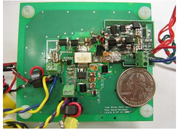
Fig. 16. Prototype dc/dc power converter.
