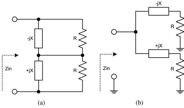
Fig. 3. Structure of some resistance compression networks. The impedance of the reactive networks is specified at the desired operating frequency. Implementation of the reactive networks may be selected to provide desired characteristics at frequencies away from the operating frequency.
