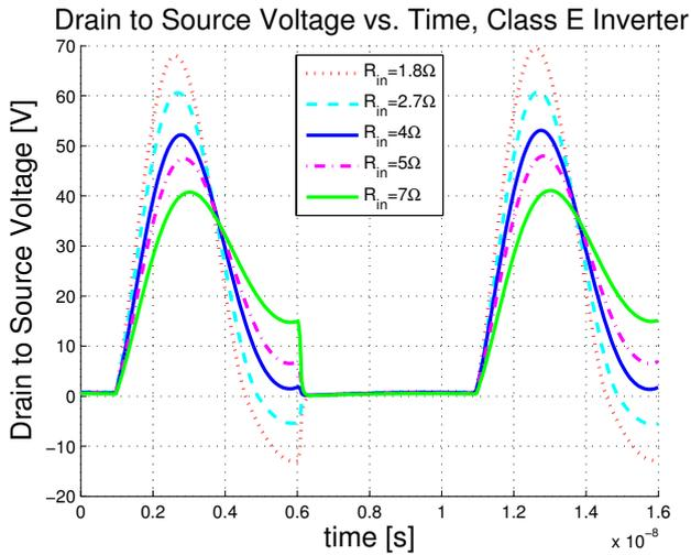
Fig. 11. Drain to source voltage for a Class E inverter for different values of resistance. Using the notation in [27]  $L_1 = 538nH$ ,  $L_2 = 24.2nH$ ,  $C_1 = 120pF$  (non-linear),  $C_2 = 163.5pF$ ,  $1.8\Omega \leq R \leq 7\Omega$ . Optimal Zero-voltage switching (ZVS) occurs at  $R = 4\Omega$ . When the resistor deviates from its nominal value ZVS is not achieved.
