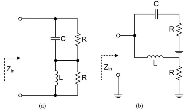
Fig. 2. Resistance compression circuits. Each of these circuits provides a compression in apparent input resistance. At the resonant frequency of the LC tank the input resistance  $R_{in}$  varies over a narrow range as the matched resistors  $R$  vary over a wide range (geometrically centered on the tank characteristic impedance). The circuits achieve lossless energy transfer from the input port to the resistors  $R$ .
