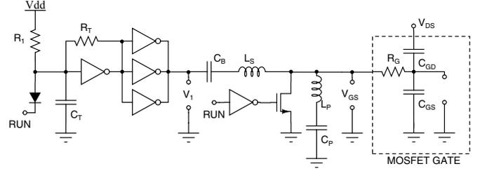
Fig. 3. Sinusoidal resonant gate drive circuit. This driver is employed in the 50 MHz converter (Figure 12).
