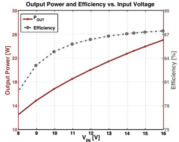
Fig. 7. Open-loop power and efficiency of the 110 MHz converter over the input voltage range for the 110 MHz converter, with  $V_{out}$  fixed at 32 V.
