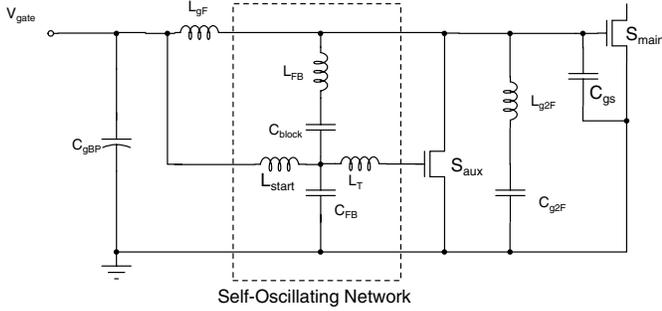
Fig. 2. Trapezoidal resonant gate drive circuit with self-oscillating network. The converter is enabled by applying the voltage  $V_{gate}$ , and disabled by setting  $V_{gate}$  to zero. This gate driver is employed in the 110 MHz converter (Figure 5).
