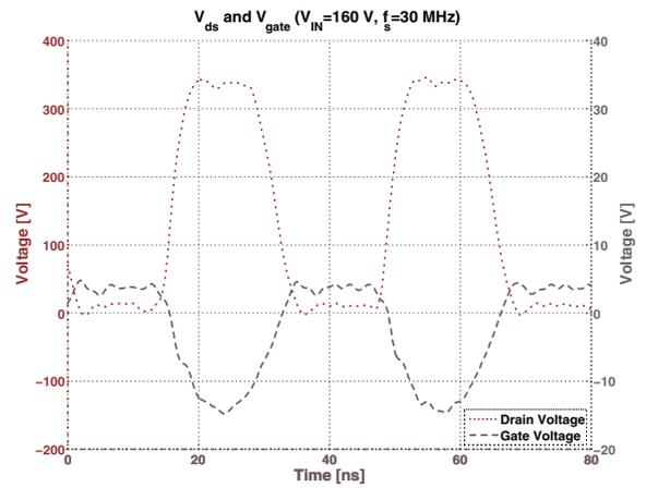
Fig. 9. Experimental MOSFET drain to source and gate voltage at  $V_{IN}=160$  V. The gate is driven from a  $50\Omega$  power amplifier through a CX2024 transmission-line transformer.
