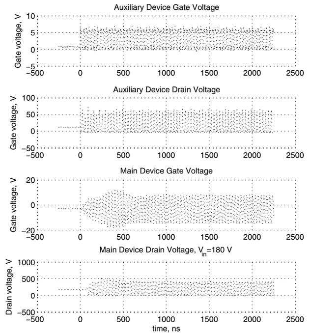
Fig. 18. Experimental turn-on transient with gate drive.  $V_{IN} = 180$  V,  $V_{bias} = -3$  V, load at or above 31 V.
