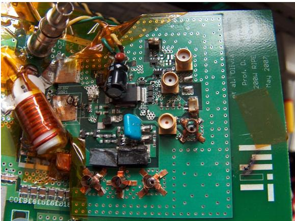
Fig. 17. Photograph of the gate drive board.
