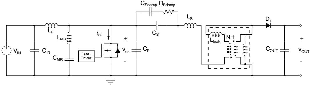
Fig. 2. Dc-dc converter as implemented with an autotransformer.
