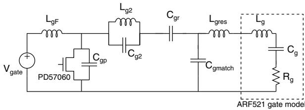
Fig. 13. Resonant second harmonic class E gate driver.
