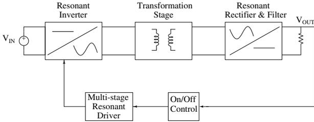
Fig. 1. General structure of the proposed dc-dc converter.
