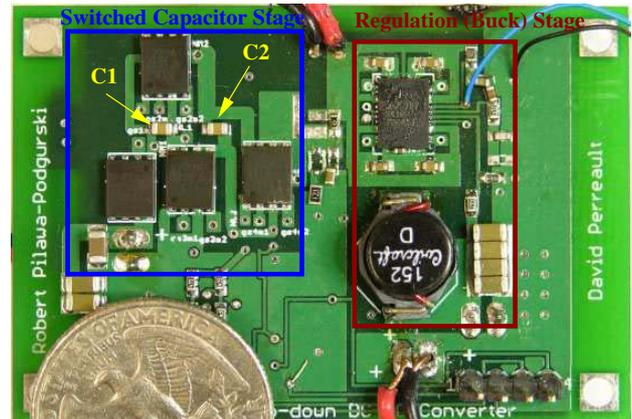
Fig. 8. Photograph of experimental prototype with switched-capacitor stage and regulation stage outlined. U.S. quarter shown for scale.
