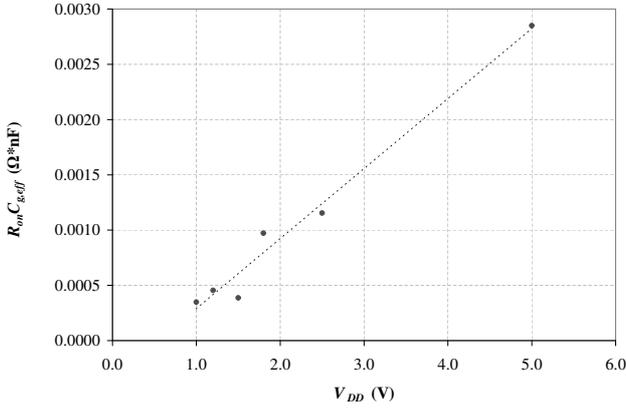
Fig. 12.  $R_{on}C_{g,eff}$  vs. Supply Voltage ( $V_{DD}$ ) for NMOS
