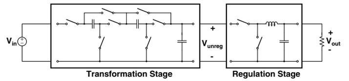
Fig. 1. Block diagram illustrating a two-stage converter. The transformation stage can be constructed using slow, high voltage devices and operated at a slow switching frequency, while the regulation stage can be constructed with fast, low-voltage devices and operated at a high switching frequency.
