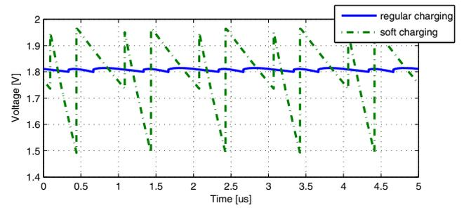
Fig. 7. Simulated output voltage waveforms ( $V_X$  of Fig. 5) for the SC converter stage, illustrating increased voltage ripple for the soft charging case.
