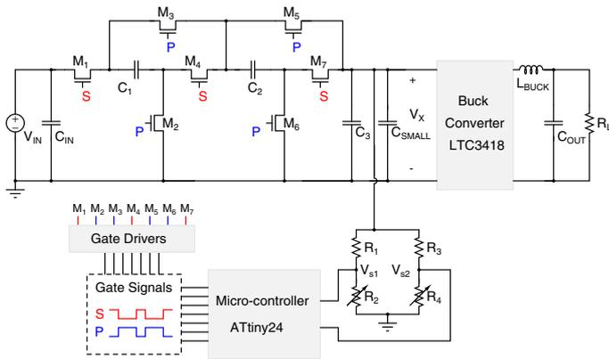
Fig. 9. Schematic of experimental prototype. The microcontroller samples the output voltage through the voltage dividers, and alternates the SC stage between parallel and series configuration.
