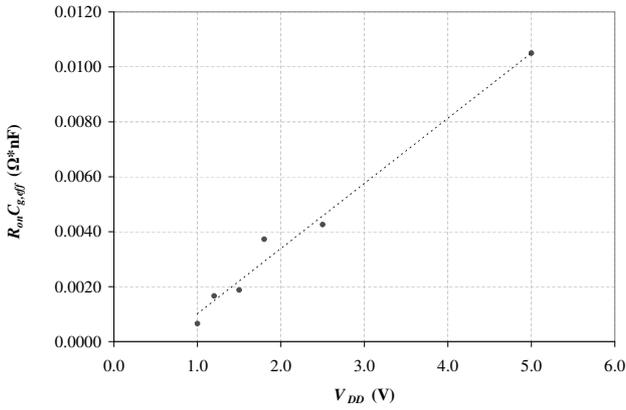
Fig. 13.  $R_{on}C_{g,eff}$  vs. Supply Voltage  $V_{DD}$  for PMOS
