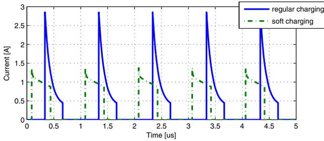
Fig. 6. Simulated current waveforms ( $I_{M1}$  of Fig. 5) for the SC converter stage, illustrating reduced peak currents (and, correspondingly, reduced loss) for the soft charging case.
