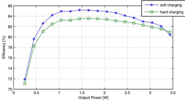
(a) Measured Overall Converter Efficiency.
