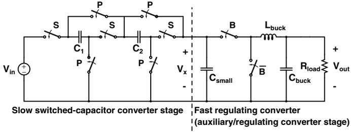
Fig. 3. Example of the switched-capacitor transformation stage circuit coupled with a fast regulating stage which provides soft charging of the switched-capacitor stage.
