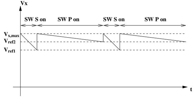
Fig. 4. Example of control strategy based on maximum input voltage of regulating converter.
