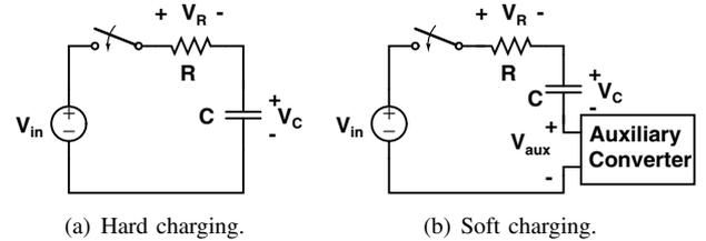
Fig. 2. Capacitor charging in a switched capacitor system. (a) Hard charging in a conventional SC system. (b) Soft charging with energy recovery.
