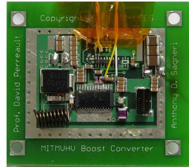
Fig. 15. A Class- $\Phi_2$  boost converter built using the MV1 device and operated to 35V. It achieves 88% conversion efficiency at 12W,  $V_{IN}=12V$ ,  $V_{OUT}=33V$ .
