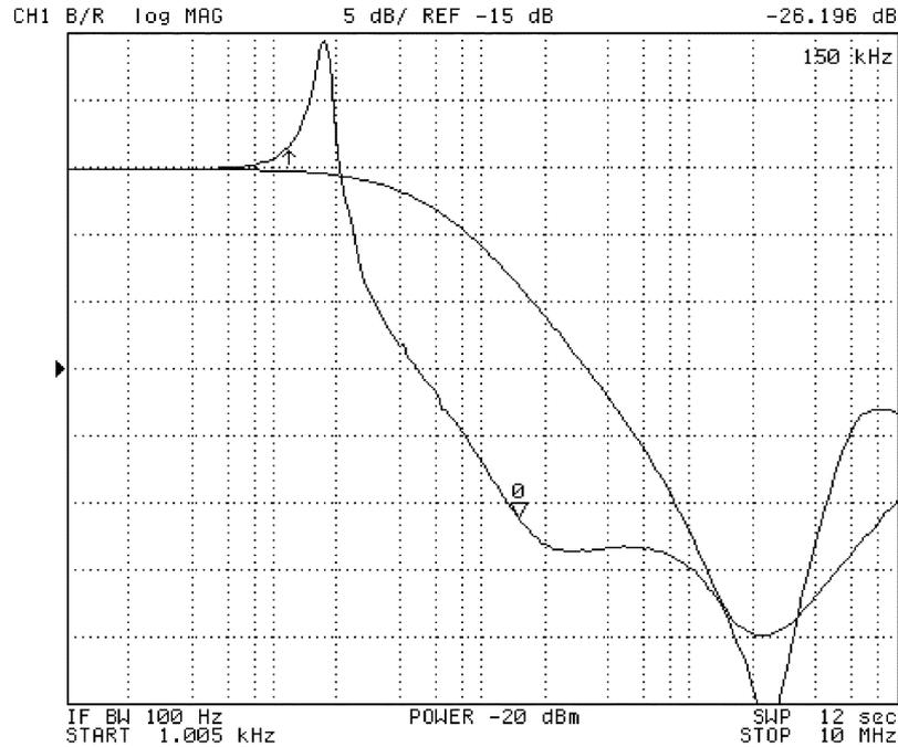
Fig. 6. System attenuation with and without active filtering for the planar design.
