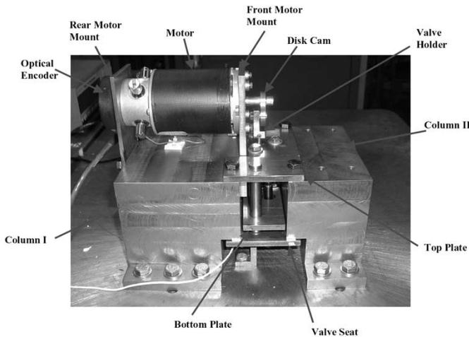
Fig. 8. Side view of the constructed EMVD apparatus.
