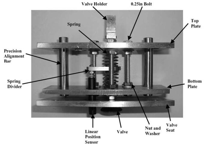
Fig. 6. Valve assembly with the soft spring set.
