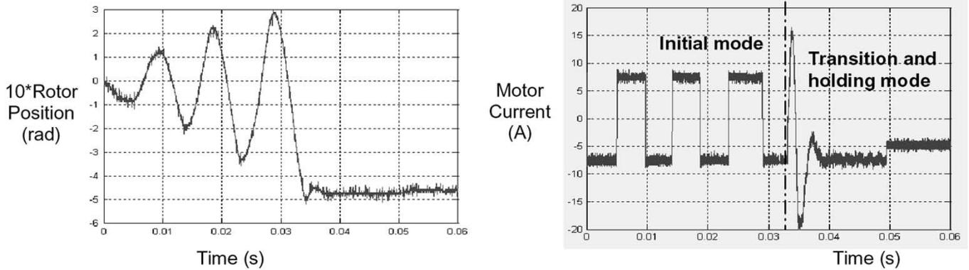
Fig. 11. Experimental waveforms during initial mode control. The initial mode transient was completed in 35 ms with  $\pm 8$  A current pulses, and required an average electrical power of 150 W.
