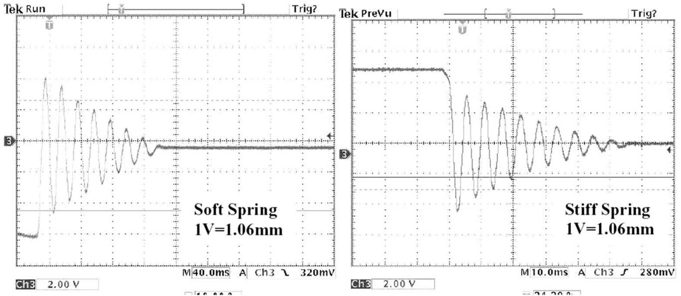
Fig. 10. Free oscillation of valve assembly with the soft and stiff spring sets.
