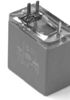
Fig. 21. Photograph of a completed 330 nF integrated filter element with inductance cancellation. The resulting package height is 1.75 mm taller than the original capacitor casing.
