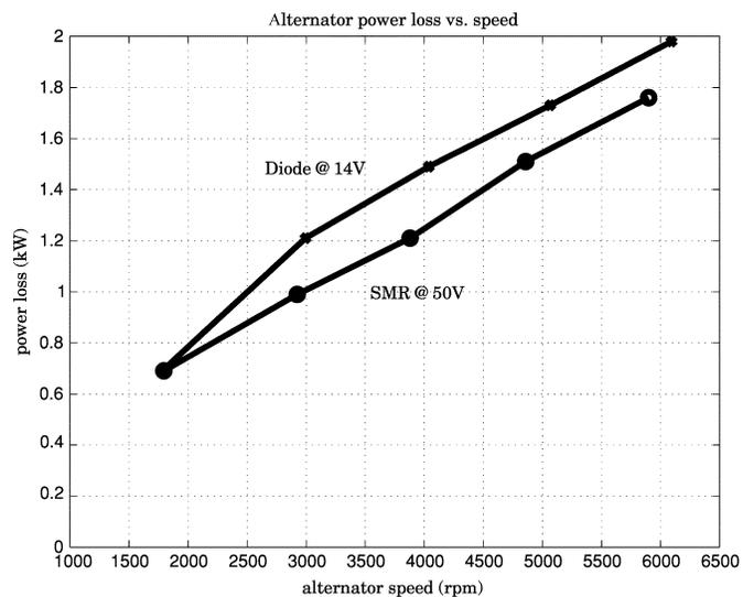
Fig. 12. Experimentally-determined alternator losses at full field across speed for different operating modes. The SMR load-matching technique (at its optimal output voltage) yields the same or lower losses than diode rectification at its optimal output voltage.
