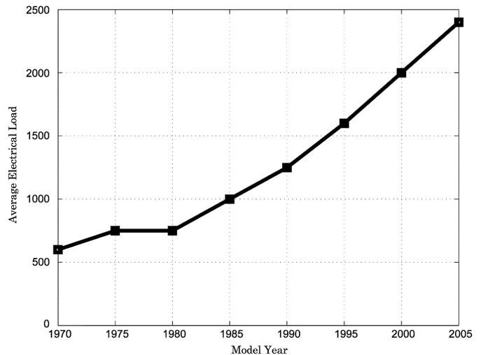
Fig. 1. Automobile electrical power requirements [1].
