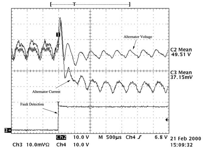
Fig. 14. Experimental demonstration of load dump transient suppression using the switched-mode rectifier (horizontal: 500  $\mu$ s/div; vertical: 10 A/div, 10 V/div).
