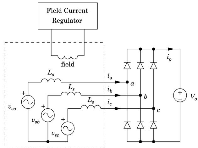
Fig. 2. Simple Lundell alternator model.
