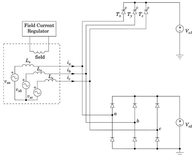
Fig. 18. Particular implementation of the dual-rectifier alternator architecture.
