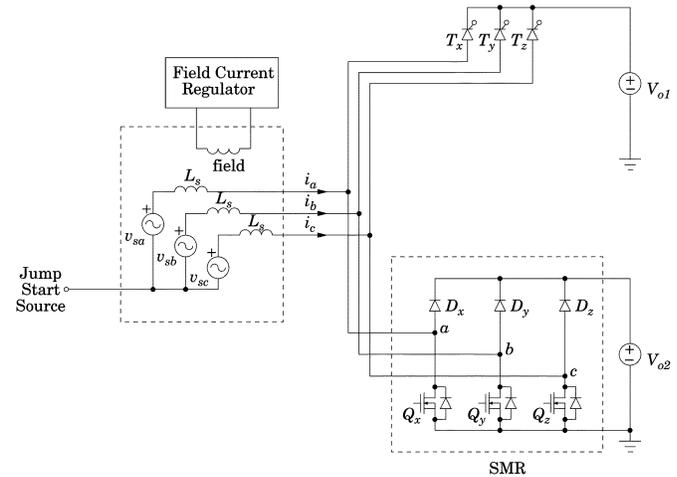
Fig. 19. Dual-rectified alternator architecture implementation using the switched-mode rectifier structure.
