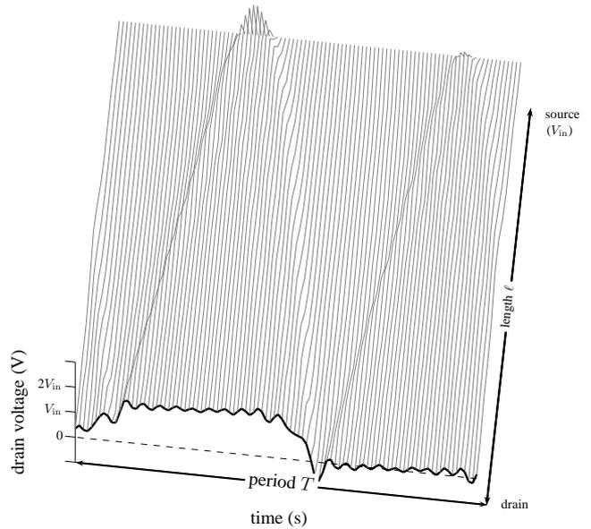
Fig. 4: Waveform symmetries (left) imposed by the  $\lambda/4$ -wave transmission line, and idealized waveforms (right) of the Class  $\Phi$  inverter built around it.
