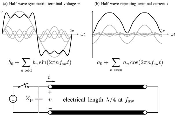
Fig. 2: Input impedance (left) of a line of length  $\ell$  terminated in a short circuit. When excited periodically at a frequency equal to the principle quarter-wave resonance, the line enforces odd- and even-harmonic symmetries in voltage and current, respectively.
