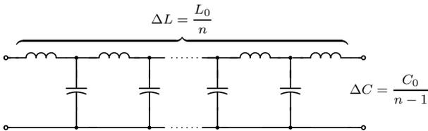
Fig. 7: Iterated Cauer model for the transmission line.
