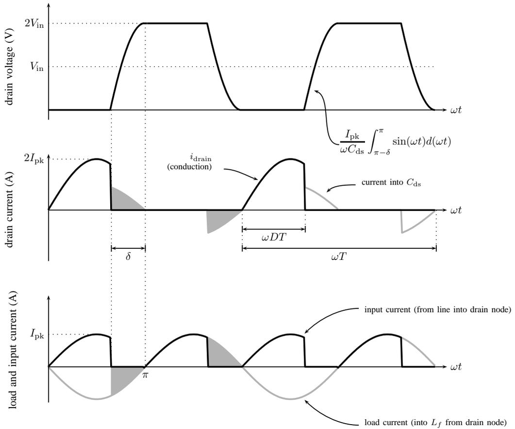
Fig. 3: Waveform symmetries (left) imposed by the  $\lambda/4$ -wave transmission line, and idealized waveforms (right) of the Class  $\Phi$  inverter built around it.
