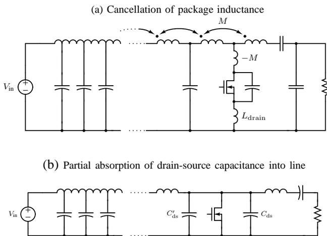
Fig. 9: Two methods of compensating for switch reactances in the Class  $\Phi$  inverter
