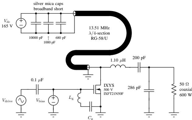
Fig. 5: Multi-resonant converter constructed with a length of RG-58/U coaxial line.
