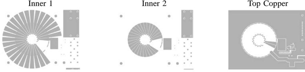
Fig. 6: Copper layers of the Class  $\Phi$  converter constructed with a lumped  $20\ \Omega$  transmission-line analog incorporated into the thickness of a PCB.
