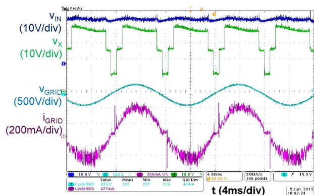
Fig. 13. Waveforms of the MEB micro-inverter, when  $V_{IN} = 27$  V,  $V_{GRID} = 230$  V<sub>rms</sub> and  $P_{OUT(ave)} = 70$  W.
