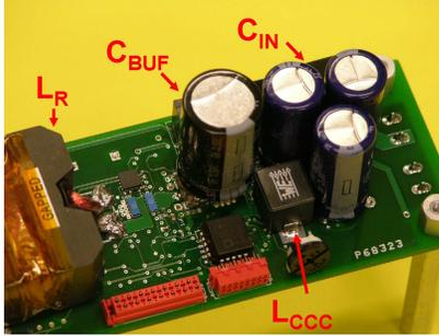
Fig. 9. Photograph of the rear side of the board showing:  $C_{IN}$ ,  $C_{BUF}$ ,  $L_{CCC}$ , and  $L_R$ .
