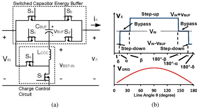
Fig. 4. One embodiment of the proposed MEB: (a) MEB circuit implementation, and (b) waveform of  $v_X$  relative to  $v_{GRID}$  during a half line-cycle.
