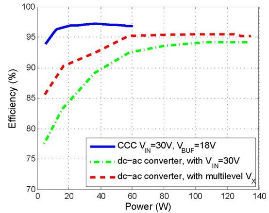
Fig. 17. Measured efficiency of the CCC, the dc-ac converter block with a fixed input voltage, and the dc-ac converter block with a multilevel input voltage when  $V_{IN} = 30$  V and  $P_{OUT(ave)} = 70$  W. The peak power rating of the dc-ac converter block is 140 W, and the peak power rating of the CCC is 65 W.
