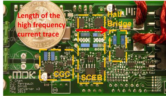
Fig. 11. PCB layout of the MEB comparing the size of the MEB and a US quarter. The area of the high-frequency current loop is minimized.
