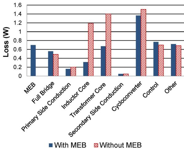
Fig. 18. Loss break-down comparison between the micro-inverter with and without the MEB, when  $V_{IN} = 30$  V and  $P_{OUT(avg)} = 70$  W.
