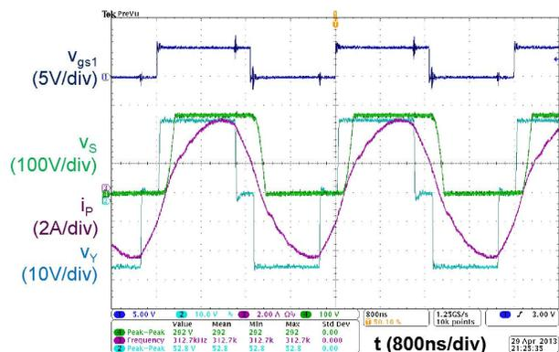
Fig. 14. Waveforms of the MEB micro-inverter showing soft-switching of  $S_1$  when the switching frequency is 312 kHz,  $V_{IN} = 27$  V,  $V_{GRID} = 230$  V<sub>rms</sub> and  $P_{OUT(ave)} = 48$  W.
