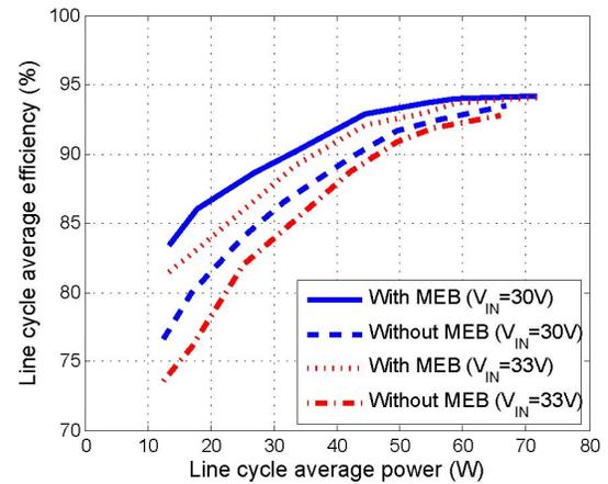
Fig. 16. Line cycle average efficiency of the microinverter with and without the MEB, with  $V_{GRID} = 230$  V<sub>rms</sub>, and  $V_{IN} = 30$  V or 33 V.
