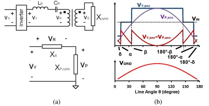
Fig. 5. (a) Model of the dc-ac converter stage. Here  $X_R$  is the impedance of the resonant tank,  $X_{cyclo}$  is the impedance of the cycloconverter (rectifier/unfolder), and  $X_{P,cyclo}$  is the impedance of the cycloconverter reflected to the primary side of the transformer. (b) Waveforms of the envelope of  $v_Y$ ,  $v_P$ ,  $v_Y - v_P$  and  $v_{GRID}$  relative to the line voltage during a half line-cycle.
