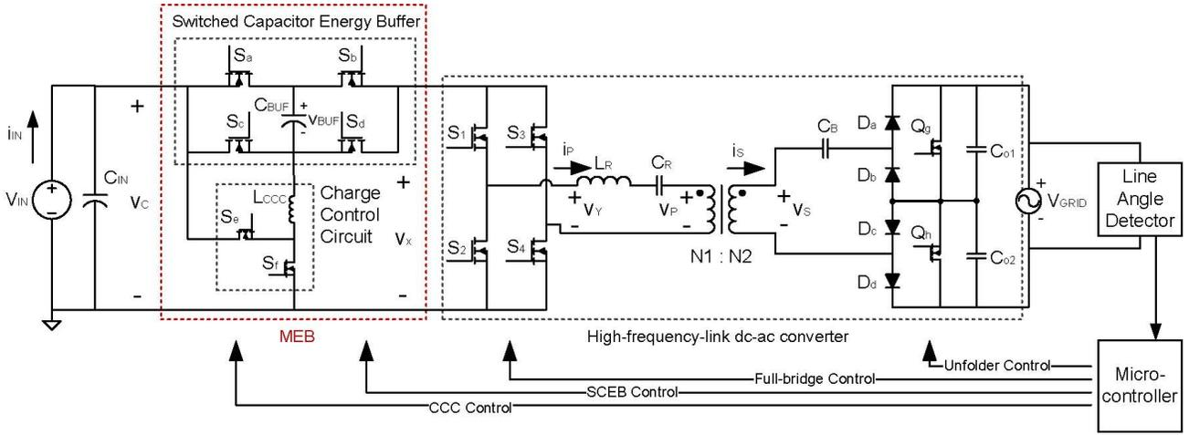
Fig. 3. One implementation of the MEB micro-inverter.
