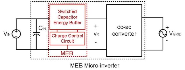
Fig. 2. Architecture of the proposed micro-inverter. It incorporates a Multilevel Energy Buffer and Voltage Modulator (MEB).
