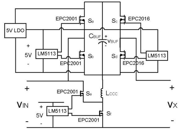
Fig. 10. Switch and gate drive implementation of the MEB.
