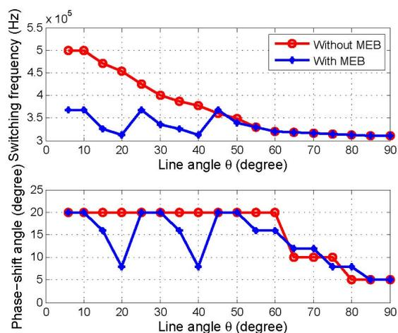
Fig. 12. Frequency and phase modulation range of the micro-inverter without and with the MEB. Range plotted for  $V_{IN} = 30$  V and  $P_{OUT(ave)} = 70$  W.
