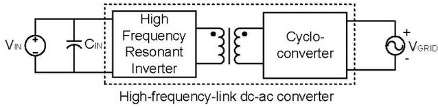
Fig. 1. Architecture of a micro-inverter incorporating a twice-line-frequency energy buffer capacitance,  $C_{IN}$ , a high-frequency resonant inverter, a transformer and cycloconverter.
