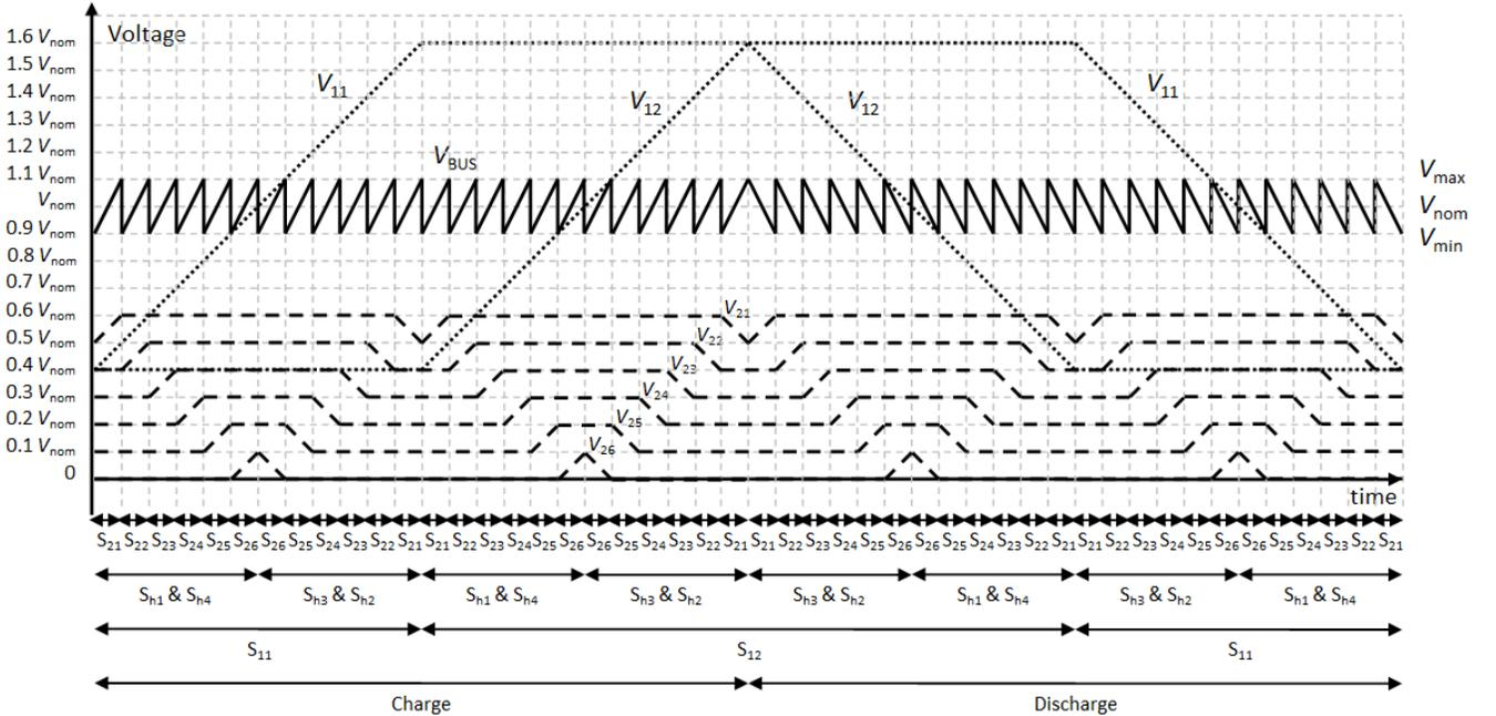
Fig. 5: Switch states, individual capacitor voltages, and resulting bus voltage over a charge and discharge cycle of the 2-6 bipolar SSC energy buffer of Fig. 4.
