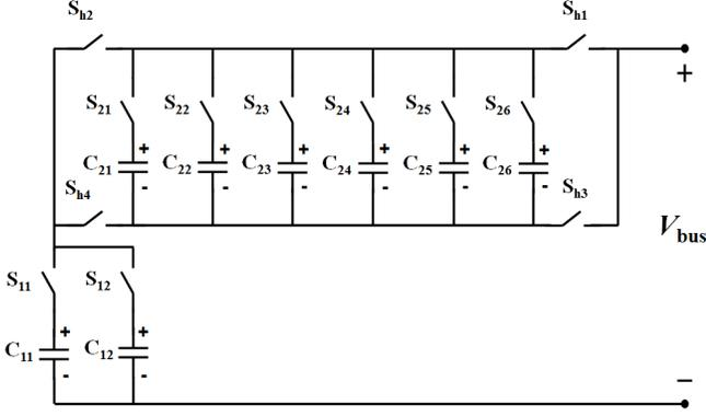
Fig. 4: An example embodiment of the SSC energy buffer architecture: the 2-6 bipolar SSC energy buffer. This circuit has two backbone capacitors  $C_{11}$  and  $C_{12}$  and six supporting capacitors  $C_{21}$  to  $C_{26}$  and twelve switches. Precharge and control circuits are not shown.
