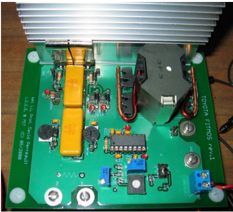
Fig. 9. This is the picture of the prototype converter. The heatsink is oversized for safety experiment purpose.
