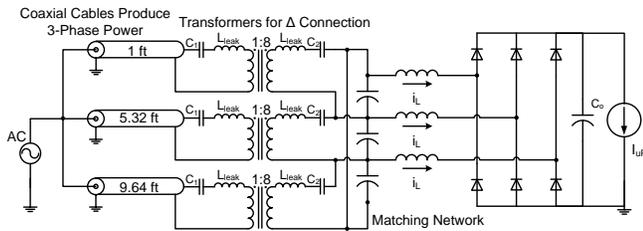
Fig. 13. Schematic of the prototype 3-phase delta-source ac power delivery system.  $C_1$  and  $C_2$  are 680 pF and 68 pF respectively. They are used for transformer leakage inductance cancellation. 68 pF ATC capacitors and 47 nH Coilcraft Midi Spring air core inductors were used to form the 3-phase delta-connected capacitor matching network.
