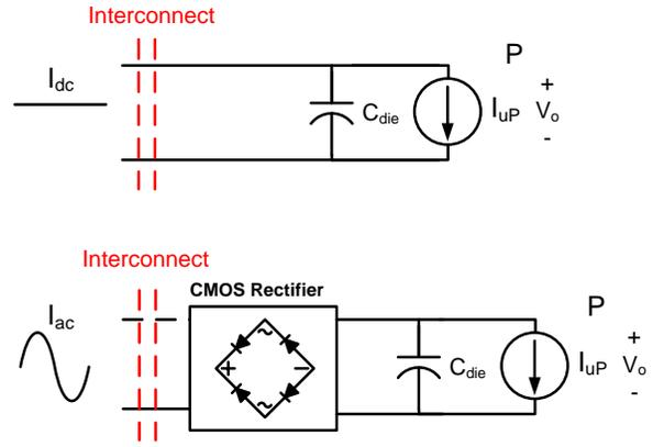
Fig. 5. System for comparison of ac and dc interconnect loss. It is assumed that each system has the same interconnect area, the same output voltage  $V_o$  and same output power  $P$ .
