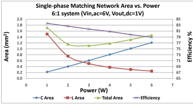
Fig. 7. This plot shows the area trade-off in the matching network for an exemplary ac power delivery system. With a given technology for passive components and voltage transformation ratio, the optimal power density of the matching network is output power dependent.
