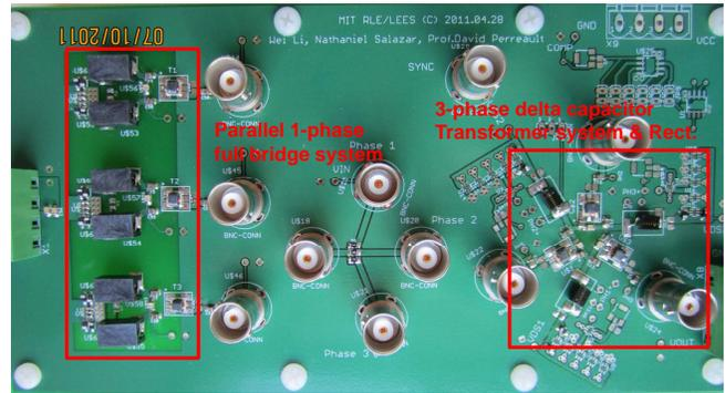
Fig. 11. Picture of the polyphase ac power delivery PCB prototype test board.
