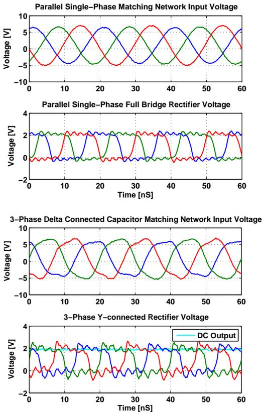
Fig. 14. Experimental results for the 3-phase 50 MHz power delivery systems. Both the system with parallel single-phase matching networks and the system with a 3-phase matching network having delta-connected capacitors shows 6 V line-to-neutral input ac voltages and 2 V dc output voltage.
