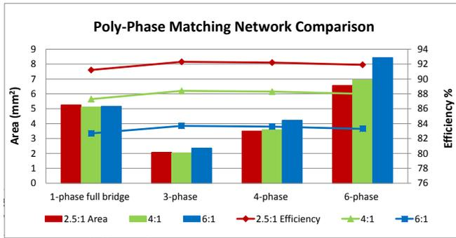
Fig. 10. Comparison of 2-W polyphase systems. The conversion ratio is the line-to-neutral voltage of the ac input to the dc output voltage. The efficiency shown is for the matching network only. The optimized rectifier performance based on IBM 65nm is about 94% in all cases. The rectifier area is about  $0.1 \text{ mm}^2$ , which is negligible compared to the rest of the system.
