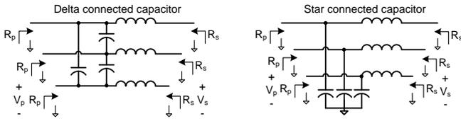
Fig. 9. This plot shows two configurations of a polyphase matching network connection. The left matching network is with delta-connected shunt elements (capacitors) and the right one is with star (“wye”/“y”) connected shunt elements (capacitors).
