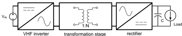
Fig. 2. General architecture of a dc-dc converter.
