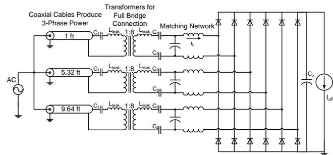
Fig. 12. Schematic of the prototype 3-phase system with separate single-phase matching networks and individual full bridge rectifiers.  $C_1$  and  $C_2$  are 680 pF and 68 pF respectively. They are used for transformer leakage inductance cancellation. 39 pF ATC capacitors and 135 nH Coilcraft Maxi Spring air core inductors were used to form the matching networks.
