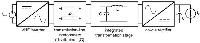
Fig. 4. Architecture of an ac power delivery system.
