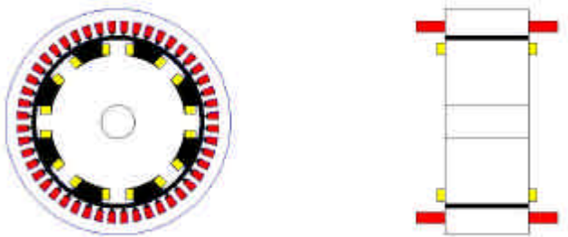
Fig. 2. Salient-pole wound-field synchronous alternator
