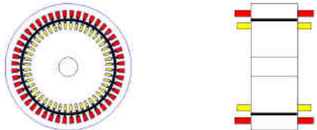
Fig. 1. Non-salient pole wound-field synchronous alternator
