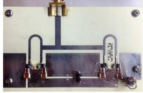
Fig. 4. Photograph of the prototype 2.45-GHz TLRCN and rectifiers.
