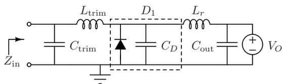
Fig. 5. Schematic of the resonant class-E rectifier used as a load for the TLRCN demonstration.
