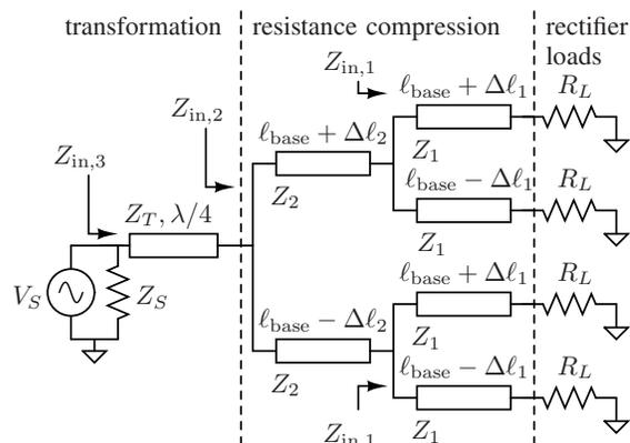
Fig. 1. Four-way TLRCN with quarter-wave impedance transformation stage. Each pair of transmission line lengths can be expressed in terms of a base line length plus and minus a delta length. The rectifiers are represented here as resistors with equal (but varying) value  $R_L$ .
