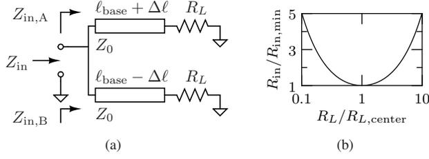
Fig. 2. Basic single-stage TLRCN and resistance compression behavior. (a) — topology, (b) — normalized input resistance vs. normalized load resistance for  $Z_0 = R_{L,center}$ ,  $\ell_{base} = \lambda/4$ , and  $\Delta\ell = \lambda/8$ .
