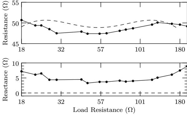
Fig. 3. Theoretical (dashed) and measured (solid) input resistance and reactance to the two-stage TLRCN when it is terminated with resistive loads. The phase of the input impedance remains within about 4 degrees over the entire 18–170  $\Omega$  operating range.
