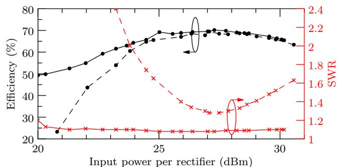
Fig. 6. Efficiency of a single rectifier (dashed), and four rectifiers plus the TLRCN (solid), including losses due to impedance mismatch. The measured SWR is also shown. Including the TLRCN substantially improves the impedance match over the entire input power range.
