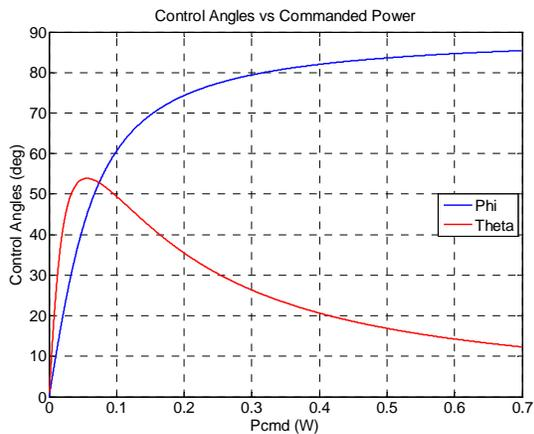
**Fig. 9** Plot showing the outphasing control angles vs. commanded output power according to (20) to (22) for the example system ( $V_s = 1$  V,  $R_L = 50$   $\Omega$ ,  $X_2 = 48.78$   $\Omega$  and  $X_1 = 35.60$   $\Omega$ ).
