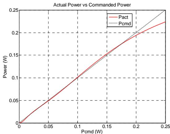
**Fig. 10** Actual output power vs. commanded power for the example system ( $V_s = 1$  V,  $R_L = 50$   $\Omega$ ,  $X_2 = 48.78$   $\Omega$  and  $X_1 = 35.60$   $\Omega$ ). The actual power increases monotonically from zero with commanded power, and matches the commanded power well over the range shown. At higher commanded power levels the actual power achieved saturates at approximately 0.31 W.
