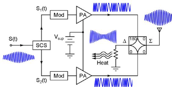
**Fig. 2** The conventional outphasing architecture implemented with an isolating combiner. A portion of the total constant output power from the PAs is delivered to the output (at the sum port of the combiner); the remainder is delivered to the difference port and is lost as heat in the isolation resistor. In some implementations, power not delivered to the output is instead recovered back to the dc supply via a rectifier.
