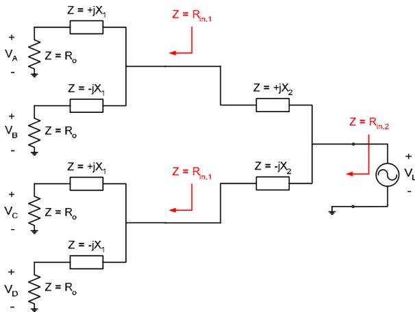
**Fig. 5** A multi-stage resistance compression network based on a cascade of the single-stage RCN network in Fig. 4. A source  $V_L$  driving the network is also shown. The input resistance  $R_{in,2}$  varies much less than the matched load resistances  $R_o$ .
