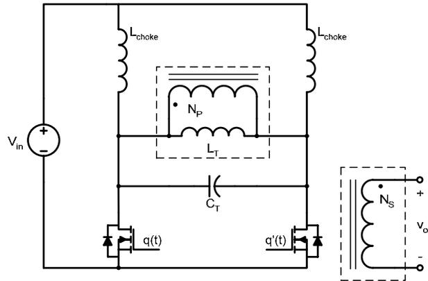
**Fig. 18** This figure shows the E/F<sub>odd</sub> power amplifier used in the example system simulations. The power amplifier is designed to operate at 27.12 MHz at an input voltage of 125 V and at output powers up to 750 W. The tank capacitor  $C_T = 96.1$  pF is selected in conjunction with the 80 pF device capacitance to be at resonance with the primary-referred magnetizing inductance of the transformer  $L_T = 195.6$  nH.
