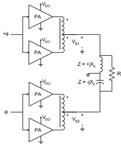
**Fig. 19** Implementation of the Chireix outphasing system. Each of the two outphased sources is constructed of from a pair of power amplifiers (of the type in Fig. 18) operated synchronously, with their outputs combined through interphase transformers. The Chireix combiner has  $X_c = 13.6$   $\Omega$  and the load resistance  $R_L = 13$   $\Omega$  (corresponding to one of the Chireix designs of Fig. 13).
