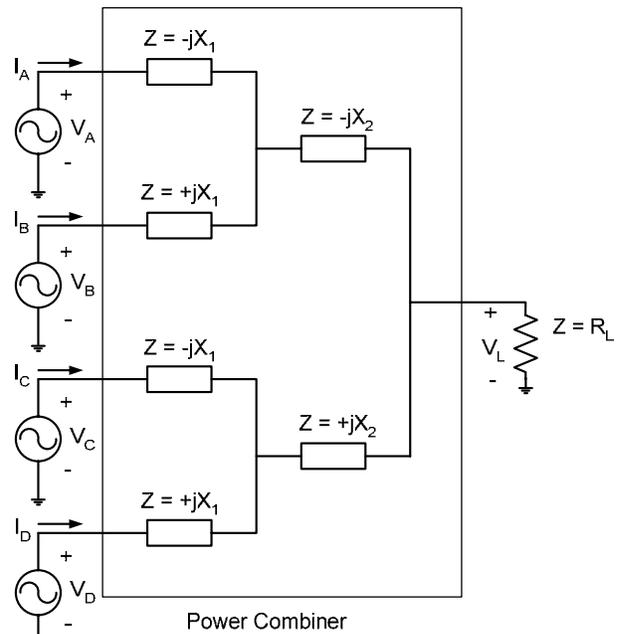
**Fig. 8** An example implementation of the proposed outphasing architecture. This implementation employs four power amplifiers (as compared to two in conventional outphasing); the power amplifiers are illustrated as ideal voltage sources in this figure for analysis purposes. The power combiner is ideally lossless, and comprises reactive elements with specified impedances at the operating frequency. The combiner has five ports: four for the power amplifier inputs and one for the load.
