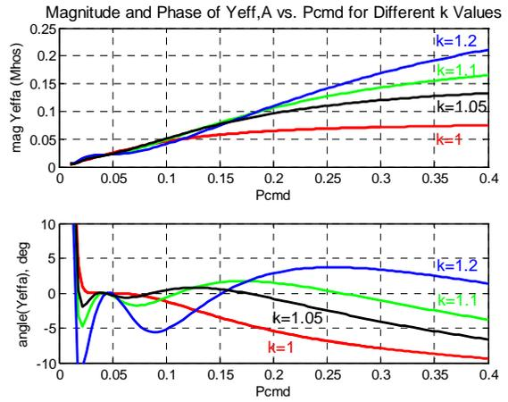
**Fig. 22** This figure shows plots of the effective admittance  $Y_{eff,A}$  in the combiner of Fig. 8 and control laws (20) – (22) for different values of design parameter  $k$ . It can be seen that higher values of  $k$  provide a higher upper bound in achievable power delivery, but also result in greater phase variations over the operating range.
