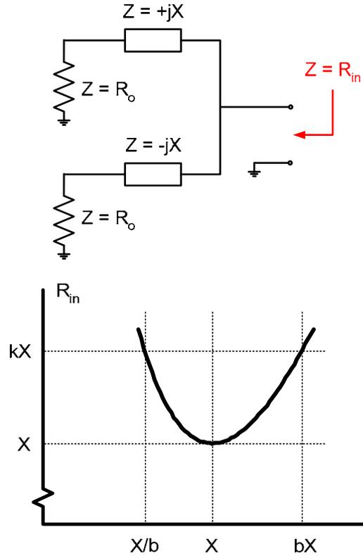
**Fig. 4** (top) A basic resistance compression network (RCN) and (bottom) its resistive input impedance  $R_{in}$  as a function of the matched load resistance value  $R_o$ . As the resistances  $R_o$  vary together over a range geometrically-centered on  $X$ , the input impedance is resistive and varies over a much smaller range than  $R_o$ . RCN networks have application to resonant dc-dc converters and rectifiers [30,31] and to energy recovery in power amplifiers [22] among other uses.
