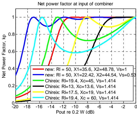
**Fig. 15** Net power factor as a function of normalized output power for four Chireix systems and for two systems of the proposed architecture. It can be seen that the proposed power combining and outphasing system provides nearly ideal power factor across a wide power range.
