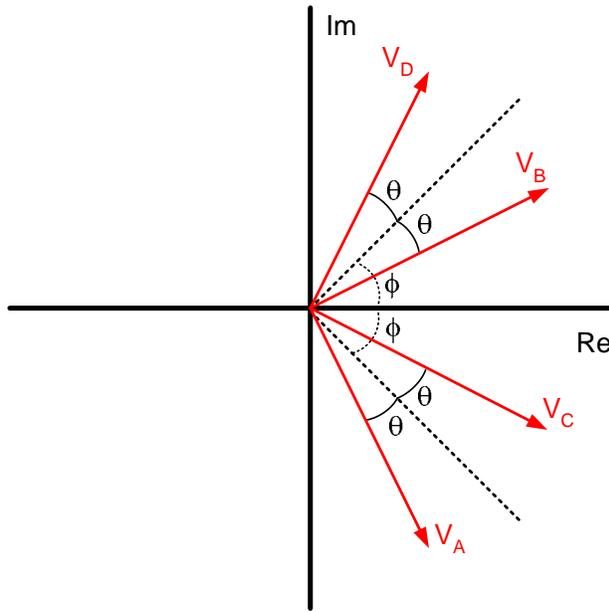
**Fig. 7** Phasor diagram showing the relationship among the phase voltages. The outphasing control angles  $\phi$  and  $\theta$  are used to regulate output power while maintaining desirable loading of the sources.
