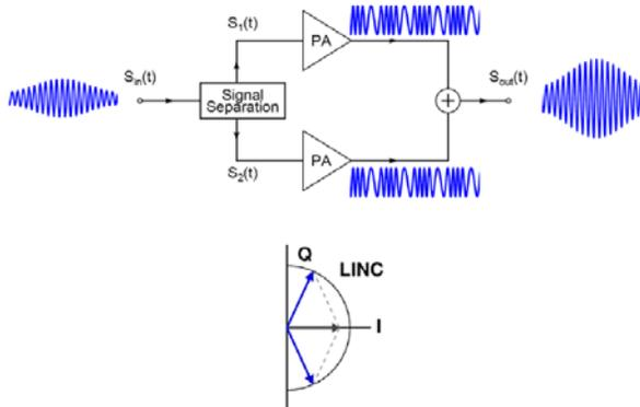
**Fig. 1** The conventional outphasing architecture, also known as the LINC architecture. A variable envelope output is created as the sum of two constant-envelope signals by outphasing of the two constant envelope signals.
