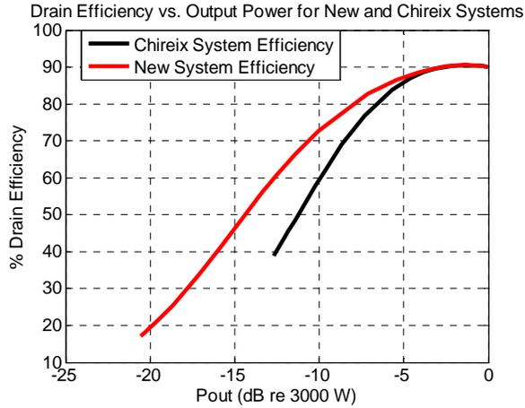
**Fig. 20** Drain efficiency vs. output power for the both the new outphasing system and the Chireix system. Efficiency is plotted over the entire outphasing range, such that this plot also indicates the output power operating ranges of the power amplifier systems.
