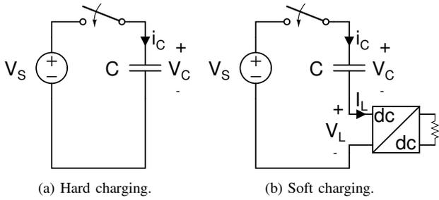
Fig. 2. Simplified circuits for illustrating capacitor charging in a switched capacitor system. (a) Hard charging in a conventional SC system. (b) Soft charging with energy recovery.
