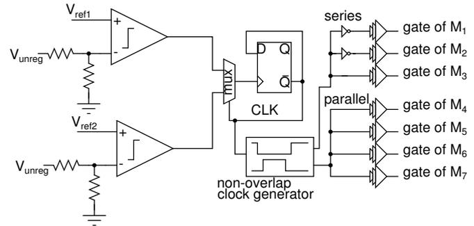
Fig. 4. The control strategy of Fig 3 is implemented using dual comparators and a flip-flop to keep state between series and parallel operation. The 5 V power mosfets (shown in the schematic of Fig. 6) are driven by level-shifted tapered gate drivers.
