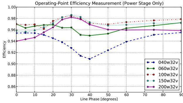
Fig. 16. Experimentally obtained power-stage conversion efficiencies for the prototype converter, at an input voltage of 32 V, over one-quarter of a line cycle.
