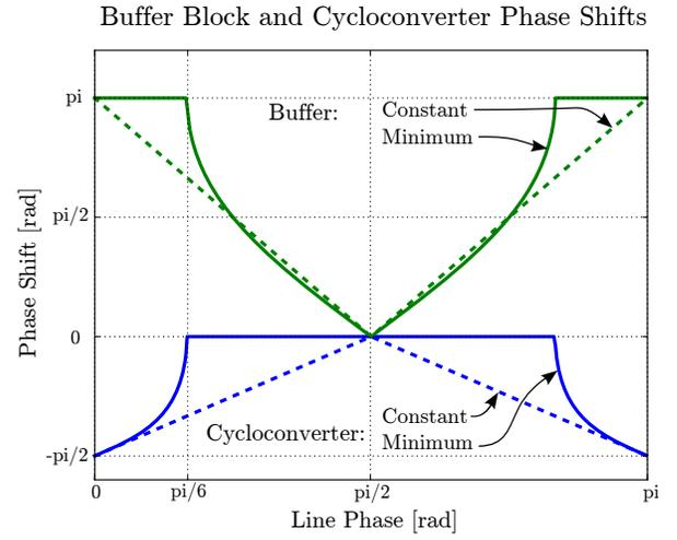
Fig. 9. The phase-modulation control parameters for the cycloconverter and buffer blocks, when operated under constant-current and minimum-current modes.
