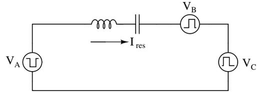
Fig. 4. The proposed topology of Fig. 3, where each active switching block is replaced with a square-wave voltage source. The applied voltage of all three blocks results in a high-frequency series current which links each block together.
