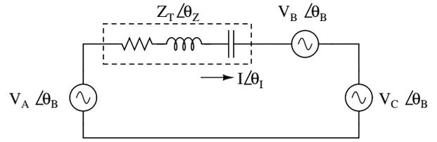
Fig. 13. The phasor equivalent of the circuit shown in Fig. 4, which approximates the operation of each active block as a sinusoidal voltage source.
