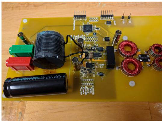
Fig. 6. Photograph of the prototype converter, including twice-line-frequency energy buffer capacitor, power stage inductor, switching and control elements, and input filter and rectifier.
