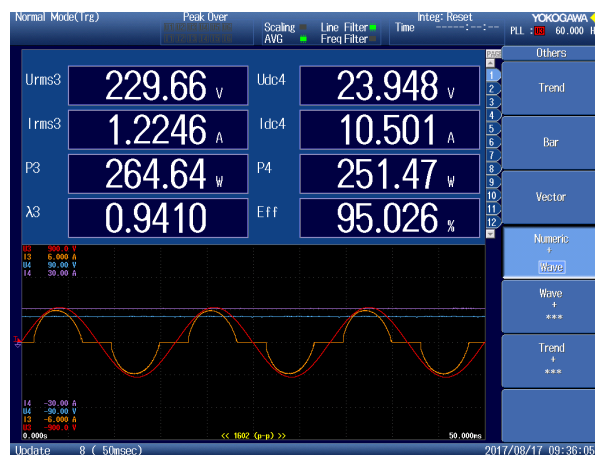
Fig. 9. Line voltage (red), line current (yellow), output voltage (blue) and output current (purple) for the following operating point: input of 230 Vac output voltage of 24 V and output power of 251 W. The power factor is 0.941 and efficiency 95.02%. The line current follows the line voltage.
