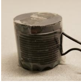
Fig. 10: Prototype inductor. Vertical windows in the outer shell were added to impede the circumferential component of flux and to allow the winding terminations to leave the structure.
