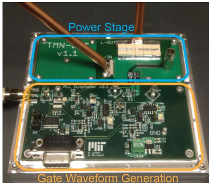
Fig. 10: Closer view of the power stage along with the gate waveform generation module. Control of the switch conduction angle is achieved through a UART serial interface.
