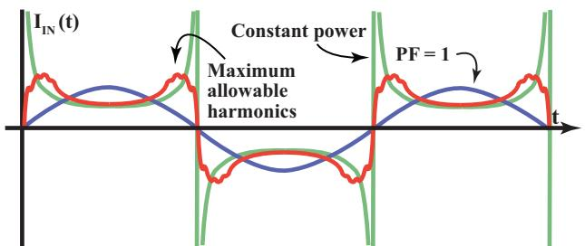
Fig. 3. Input current waveforms for  $\text{PF} = 1$  (blue), zero-buffer solution (green), and maximum Class D harmonic current (red). The maximum harmonic current waveform closely approximates the zero-buffer current for a large portion of line cycle.
