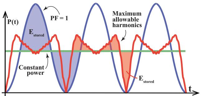
Fig. 4. The energy storage requirement when using maximum allowable Class D harmonics (shaded area, red) is significantly decreased from the energy storage required at  $\text{PF} = 1$  (shaded area, blue).
