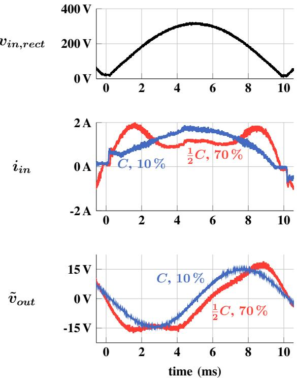
Fig. 16. Comparison of output voltage ripple when harmonics are included (10% vs 70% of the allowable third and fifth harmonics) and capacitance is reduced. The reduced voltage ripple of about 50 % in Fig. 14 is traded for 50 % less capacitance.
