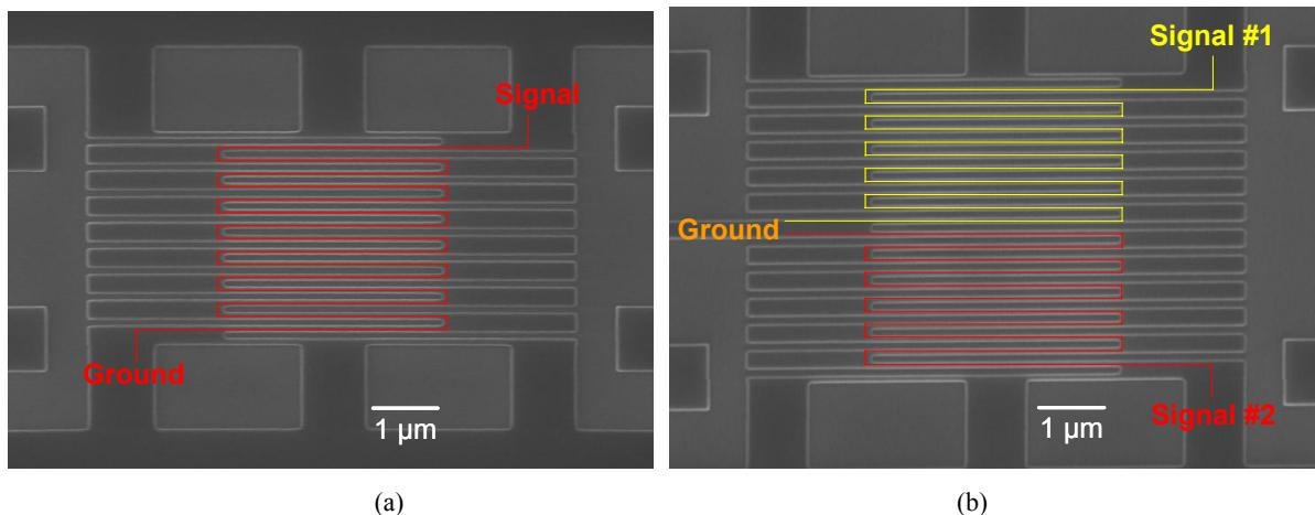
Fig. 1. (a) Scanning-electron microscope (SEM) micrograph of a 3- $\mu$ m by 3.3- $\mu$ m active area SNSPD with an overlaid path showing the flow of current from the signal contact to the ground contact. (b) SEM micrograph of a 2-element SNSPD with a 4- $\mu$ m by 4.2- $\mu$ m total active area with an overlaid path showing the flow of current in each of the detector elements.
