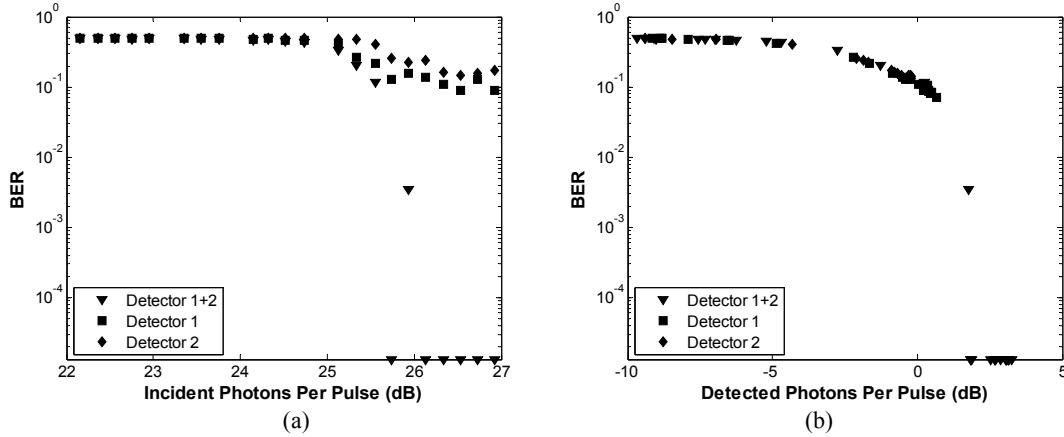
Fig. 5. Measured communications performance using 32-ary PPM at 10 Gslot/s with a  $\frac{1}{2}$ -rate turbo code (781 Mbit/s) and a 4- $\mu\text{m}$  by 4.2- $\mu\text{m}$  two-element SNSPD. Bit-error-rate performance plotted versus (a) incident photons per pulse and (b) detected photons per pulse.
