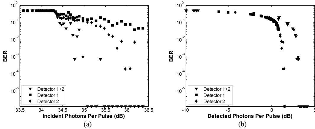
Fig. 6. Measured communications performance using 16-ary PPM at 10 Gslot/s with a  $\frac{1}{2}$ -rate turbo code (1.25 Gbit/s) and a 3- $\mu\text{m}$  by 3.3- $\mu\text{m}$  two-element SNSPD. Bit-error-rate performance plotted versus (a) incident photons per pulse and (b) detected photons per pulse.
