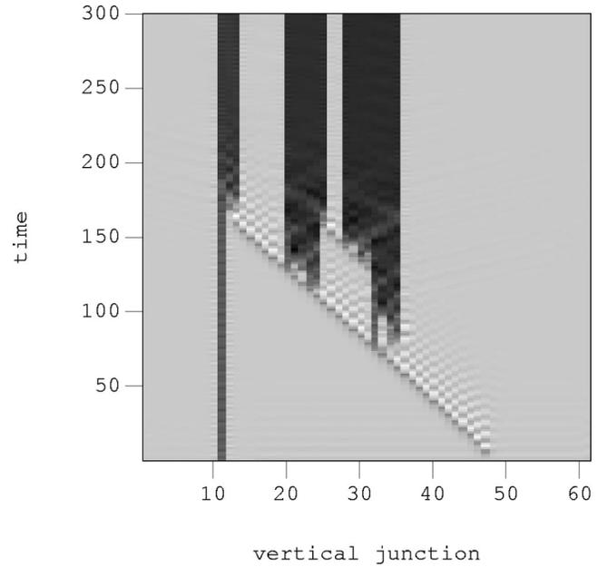
FIG. 6. Vertical junction instantaneous voltage plot of a single vortex colliding with a breather ( $i_{\text{ext}}=0.5$ ). The moving vortex switches some of the vertical junctions to rotate. The final state shows three multisite DB's with three, six and eight vertical rotating junctions, respectively.
