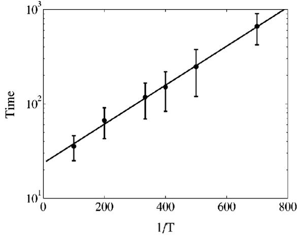
FIG. 10. Escape time for the vortex as a function of  $1/T$ . The slope of  $E_a=0.0048$  is the activation energy. Error bars represent distribution of times within one standard deviation of the mean value.
