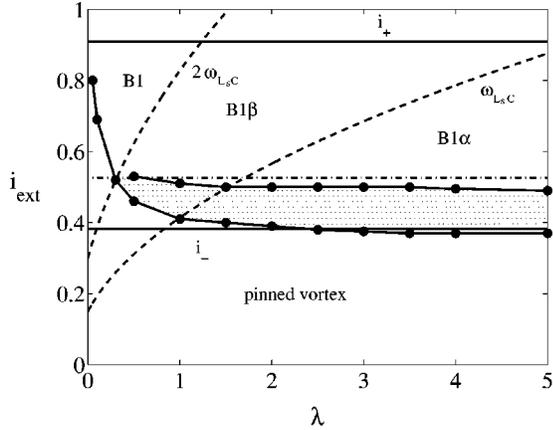
FIG. 3. Existence region of our type of breathers and a single vortex. The hatched region represents the space where a ladder supports a single traveling vortex for  $h=0.5$  and  $f=0.3$ . The dashed lines are  $\omega_{L_sC}$  and  $2\omega_{L_sC}$ .
