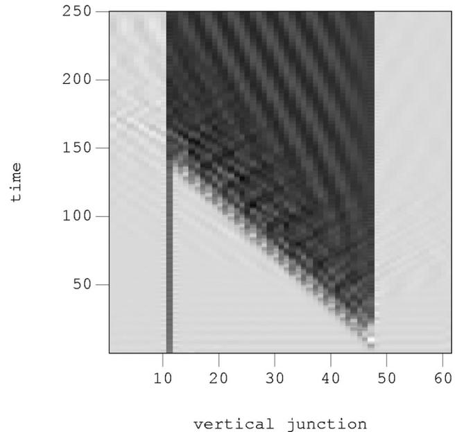
FIG. 7. Vertical junction instantaneous voltage plot of a single vortex colliding with a breather ( $i_{\text{ext}}=0.55$ ). The moving vortex switches all of the vertical junctions to rotate. In the final state all the vertical junctions between the initial position of the vortex and the breather are in the whirling state, while the others are in the superconducting state.
