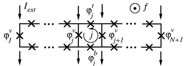
FIG. 1. The anisotropic ladder array with uniform current injection. Vertical junctions (with superscript  $v$ ) have critical current  $I_{cv}$  and horizontal junctions (with superscript  $t$  and  $b$ ) have a critical current  $I_{ch}$ .
