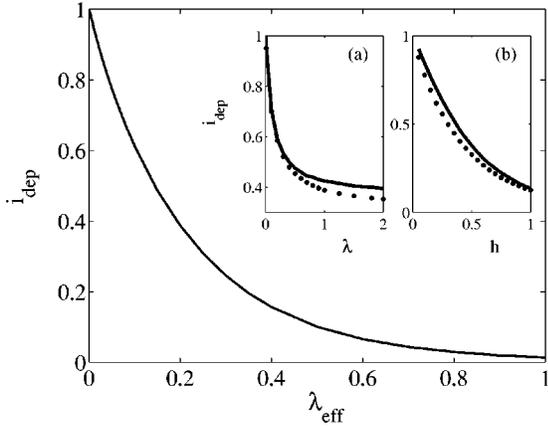
FIG. 15. Depinning current for a sine-Gordon equation as a function of the square of the penetration depth ( $\lambda_{\text{eff}}$ ). Solid circles in insets (a) and (b) are numerically calculated depinning currents of ladder when (a)  $h=0.5$  and (b)  $\lambda=5$ . Solid lines are from the sine-Gordon equation using the  $\lambda_{\text{eff}}$  value.
