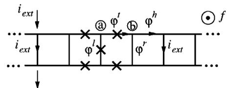
FIG. 12. Breather circuit diagram. The rotating junctions are marked by an “ $\times$ ”: other quiet junctions are marked by shorts. All of the vertical junctions in the array are biased by the external current.
