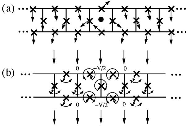
FIG. 2. (a) Sketch of a single-vortex configuration in the ladder at  $f=0$  and  $I_{\text{ext}}=0$ . In the absence of an external field this configuration is stable only at small values of  $\lambda$ . (b) Sketch of the single-site DB studied in the paper. The ladder is biased by a dc external current and one vertical and four horizontal junctions rotate while the others librate.
