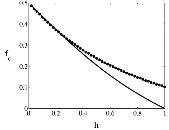
FIG. 14. Critical field needed to allow a single vortex to exist in a ladder. Solid circles are numerically calculated from full ladder dynamics with  $\lambda = 5$ . Solid line is the theoretical result from Eq. (A3).
