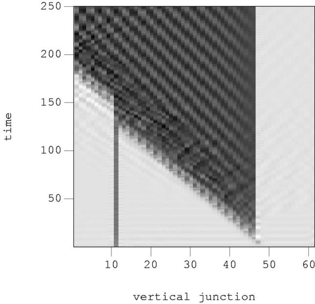
FIG. 8. Vertical junction instantaneous voltage plot of a single vortex colliding with a breather ( $i_{\text{ext}}=0.59$ ). The vortex switches all of the vertical junctions in its wake and annihilates the breather.
