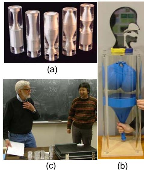
Figure 2. (a) Arai’s models of human vocal tract as educational tools. (b) A model for nasalized vowel /a/ with a lung model. (c) Arai’s models used in a class by Stevens.
