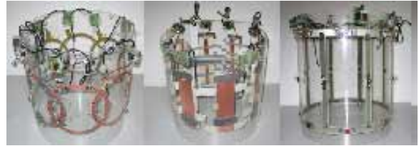
Fig 1: Parallel Transmit coils, the constructed overlapped loop coil, stripline coil and the degenerate birdcage coil (left to right).
