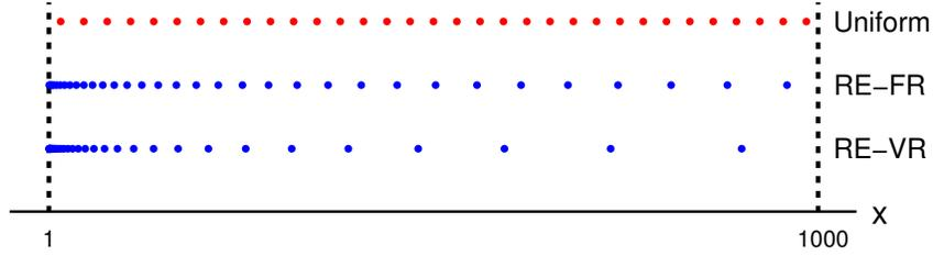
Fig. 3: Codebooks for fixed-rate and variable-rate quantizers optimized for relative error using a source uniformly distributed on  $[1, 1000]$ , as well as for a uniform quantizer, which would be optimal if the cost was MSE. The relative-error quantizers have finer quantization for smaller magnitude since the scaled error will be greater. The two variable-rate quantizers only depend on the support of the source, not its distribution.
