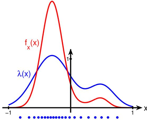
Fig. 2: An example of a source probability density function and the corresponding optimal point density function for fixed-rate quantization, defined as  $\lambda_{\text{mse,fr}}^*(x) \propto f_{\mathbf{x}}^{1/3}(x)$ . A quantizer with  $K = 21$  is represented by the dots corresponding to the placement of codewords.
