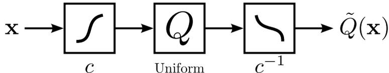
Fig. 1: A companding model for nonuniform quantization. The input  $\mathbf{x}$  is transformed by a nonlinear function  $c$  and then uniformly quantized. The nonlinearity is then inverted to produce the output  $\tilde{Q}(\mathbf{x})$ , with tilde indicating that the quantizer is generated using the compander model.
