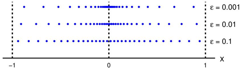
Fig. 5: Codebooks for variable-rate quantization optimized for generalized relative error when the source has support on  $[-1, 1]$ .
