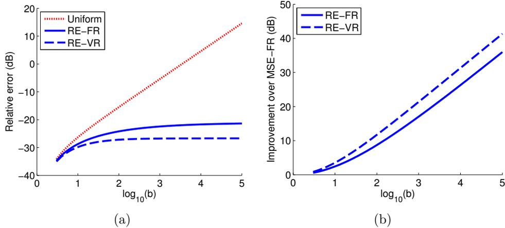
Fig. 4: Performance results of the fixed- and variable-rate quantizers with a uniform source  $\mathbf{x} \sim \mathcal{U}(1, b)$ . The plots provide trends in terms of (a) relative error in dB for  $R = 6$ ; and (b) performance gain over the uniform quantizer. The performance gain does not depend on rate.
