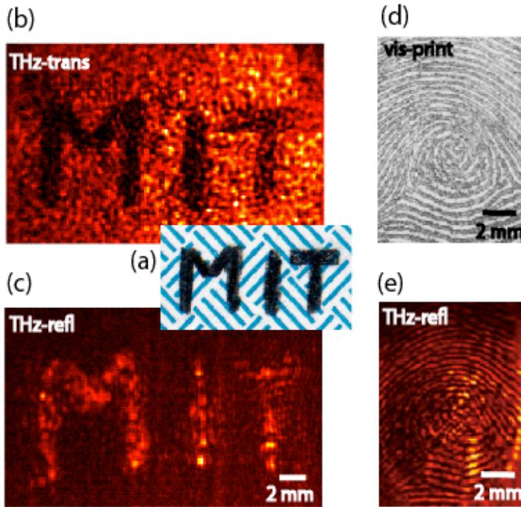
Fig. 6. Pencil letters written on the inside of a paper security envelope at visible frequencies (a), in THz transmission mode (b, 1 frame, 1/20 second) and THz reflection mode (c, 20 frames, 1 second). Visible frequency thumb print (d), and THz reflection mode image the thumb of the leading author (e, 20 frames).
