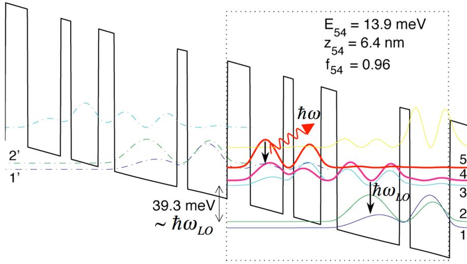
Figure 1. Conduction band profile calculated using a self-consistent Schrödinger and Poisson solver biased at 64 mV/module.
