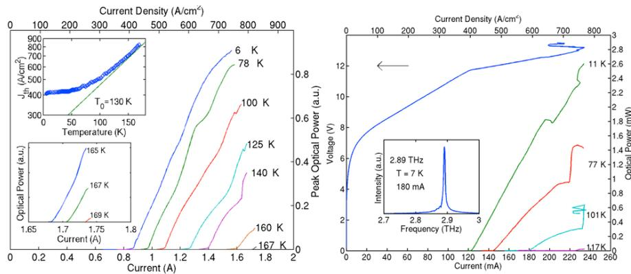
Figure 3. Left: Pulsed power-current and voltage-current relations measured up to  $\sim 169$  K heatsink temperature. Right: CW power-current and voltage-current relations measured up to  $\sim 117$  K heatsink temperature. The inset shows the CW voltage-current and differential resistance-current relations of the device.
