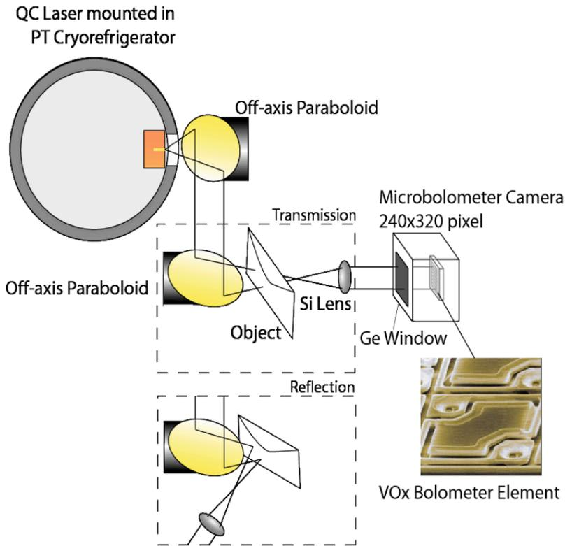
Figure. 5. Experimental setup of the THz imaging system. The photo shows a vanadium oxide microbolometer (Courtesy of BAE Systems, Lexington, MA). Cutaway depicts alternate reflection mode setup.
