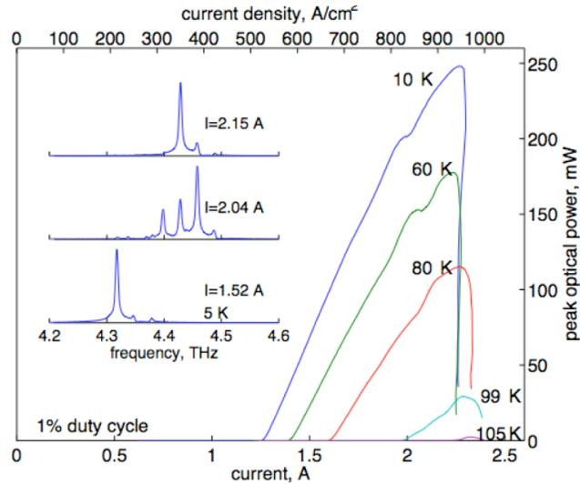
Figure 4. A ~4.4-THz quantum-cascade laser with peak power level of ~250 mW.
