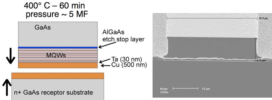
Figure 2. Left: Schematic of the wafer bonding process for double-side metal-metal waveguide. Right: A SEM picture of the fabricated device.
