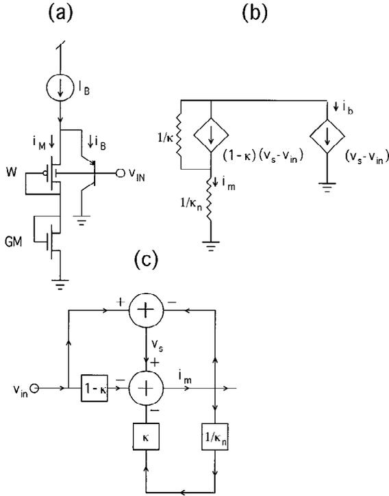
Figure A.2. The parasitic bipolar half circuit. (a) A simplified half circuit for our amplifier that is important for understanding the bipolar–mos interaction in it. (b) The small-signal equivalent circuit for (a). (c) A signal-flow diagram for the small-signal equivalent circuit.
