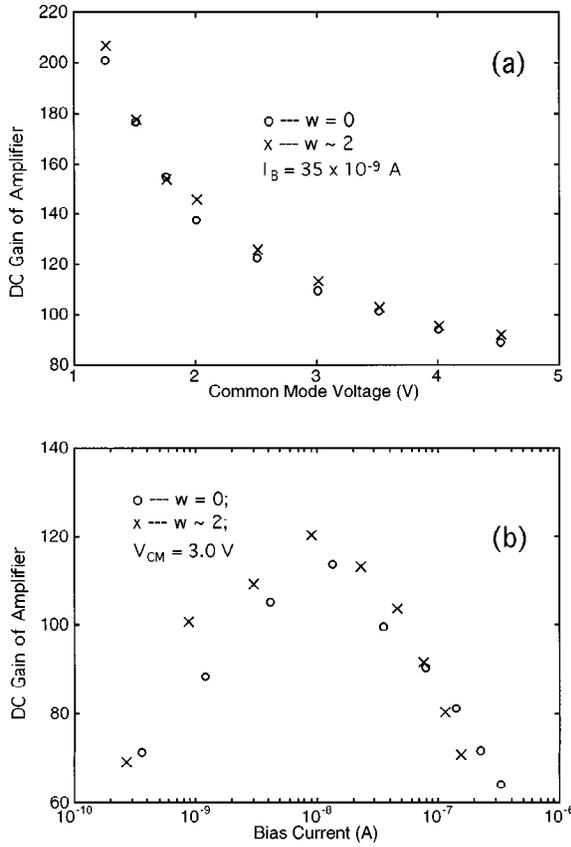
Fig. 9. Gain characteristics. (a) The gain of our amplifier as a function of the common-mode voltage. At low common-mode voltages, the gain increases because of the rising transconductance of the amplifier. (b) The gain of our amplifier as a function of the bias current. Initially, the gain rises because of the increasing Early Voltage of the amplifier, and then falls because of the increasing linear range. A more detailed discussion may be found in Section 3.3.
