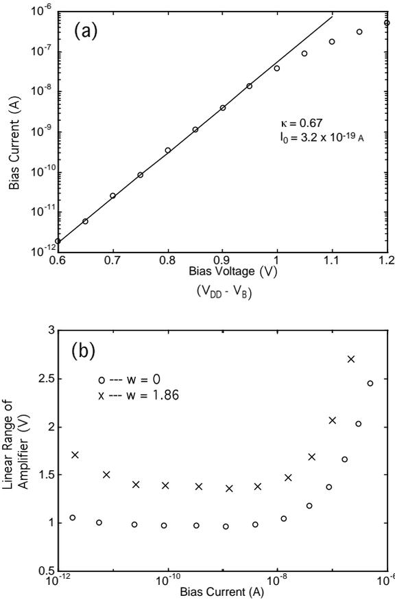
Fig. 7. Linear range vs. bias current. (a) The bias current  $I_B$  as a function of the bias voltage  $V_B$ . (b) The linear range of the amplifier  $V_L$  as a function of the bias current  $I_B$ .
