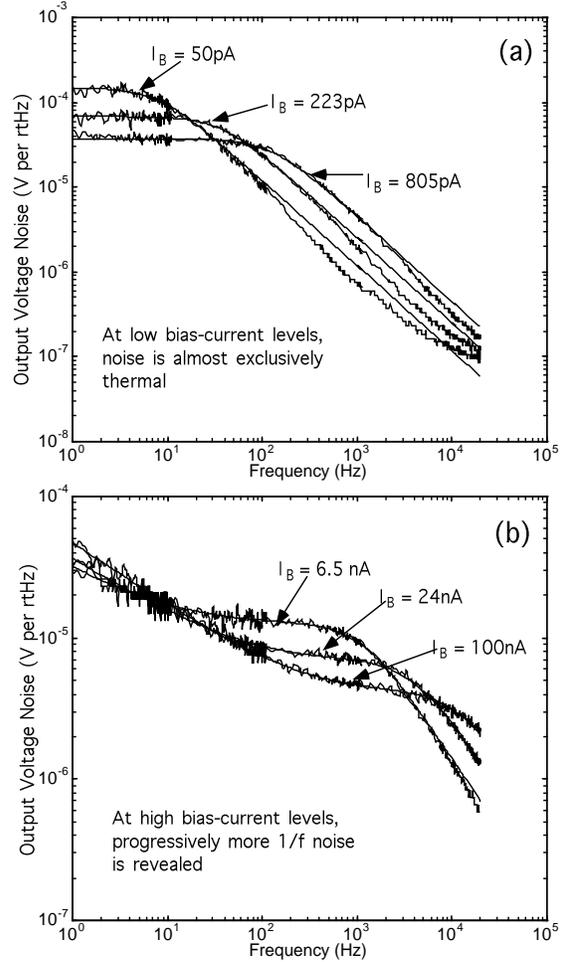
Fig. 17. Noise spectra at various current levels. (a) At low bias currents the noise is almost solely white or thermal. The bold lines are lowpass-filter fits to the data. (b) At high bias currents, there is relatively more  $1/f$  noise. Nonetheless, the dominant contribution to the noise, which is the area under this curve in a linear-linear plot, remains thermal. The bold lines are fits to the sum of a  $1/f$  term and a white-noise term.
