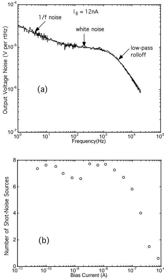
Fig. 18. Basic noise characteristics. (a) A typical noise spectrum. (b) The effective number of transistors contributing shot noise in our circuit as a function of the bias current. As the bias current goes above threshold, the effective number of transistors contributing shot noise decreases because of space-charge smoothing.
