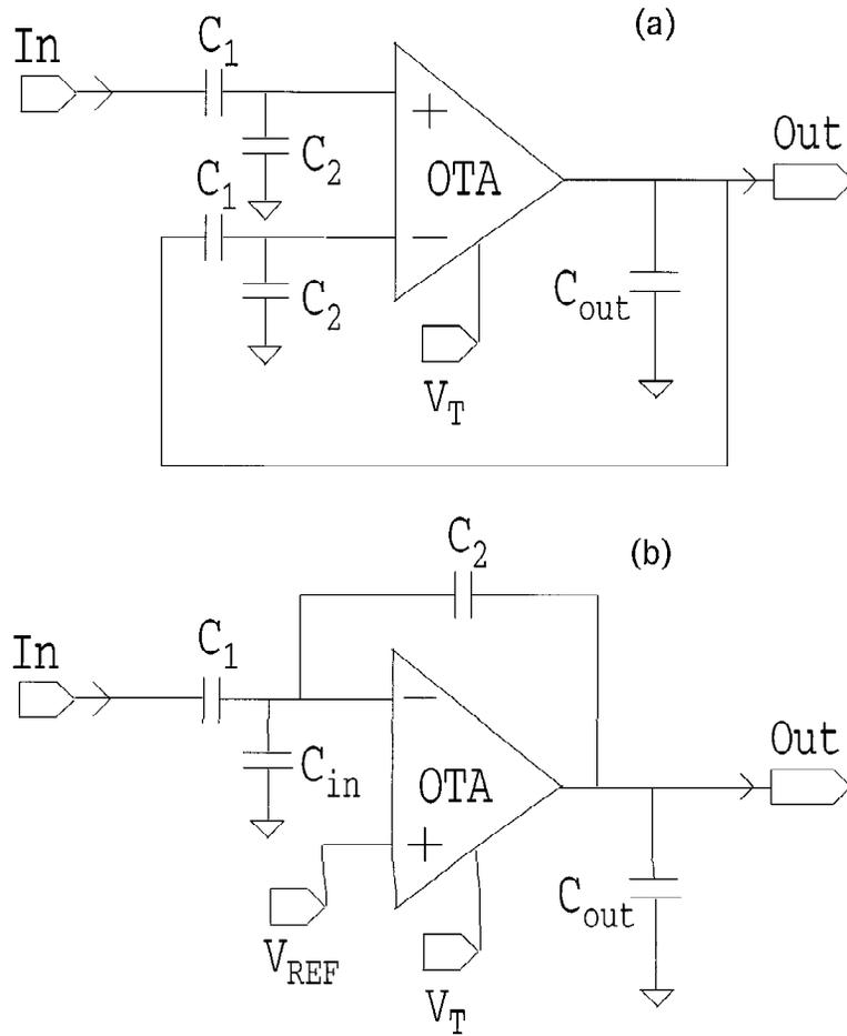
Fig. 20. Capacitive-divider schemes for widening the linear range. (a) and (b) show two different schemes. Section 5.4 contains further details.
