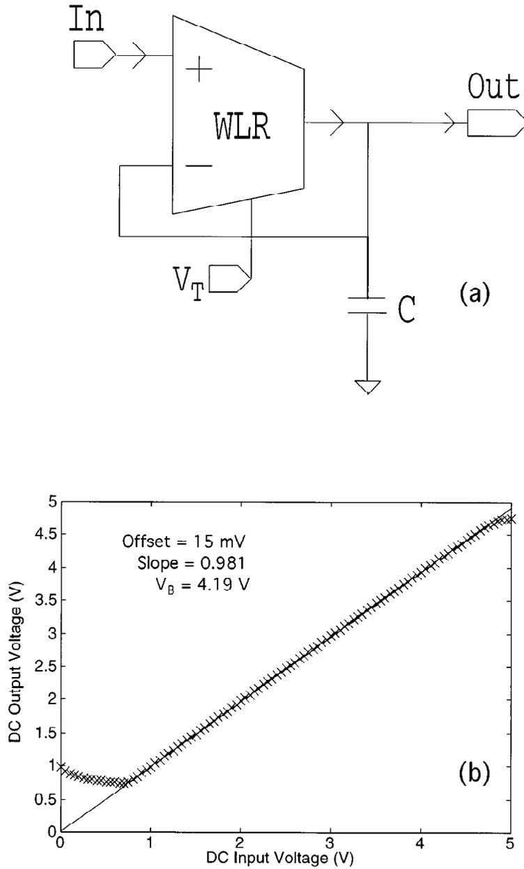
Fig. 11. Follower DC characteristics. (a) The basic circuit for a follower-integrator. (b) The output is a faithful replica of the input except at very low input voltages.
