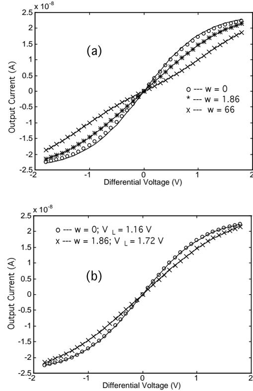
Fig. 4. I–V curves for the amplifier. (a) Experimental data for our amplifier for values of  $w = 0, 1.86,$  and  $66$ , fitted to Eq. (19). (b) For  $w \approx 2$ , the simple tanh-fit of Eq. (16) is a good approximation to Eq. (19), if  $V_L \rightarrow (3/2)V_L$ .
