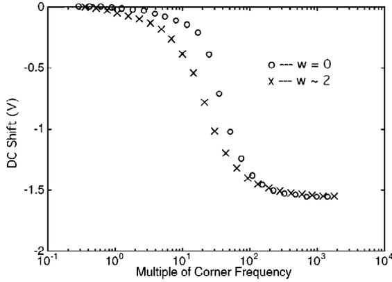
Fig. 15. DC shifts in the follower-integrator. The shifts are shown at an input rms amplitude of 1V. These shifts exert only a mild influence in cochlear designs. See Section 4.1 for details.
