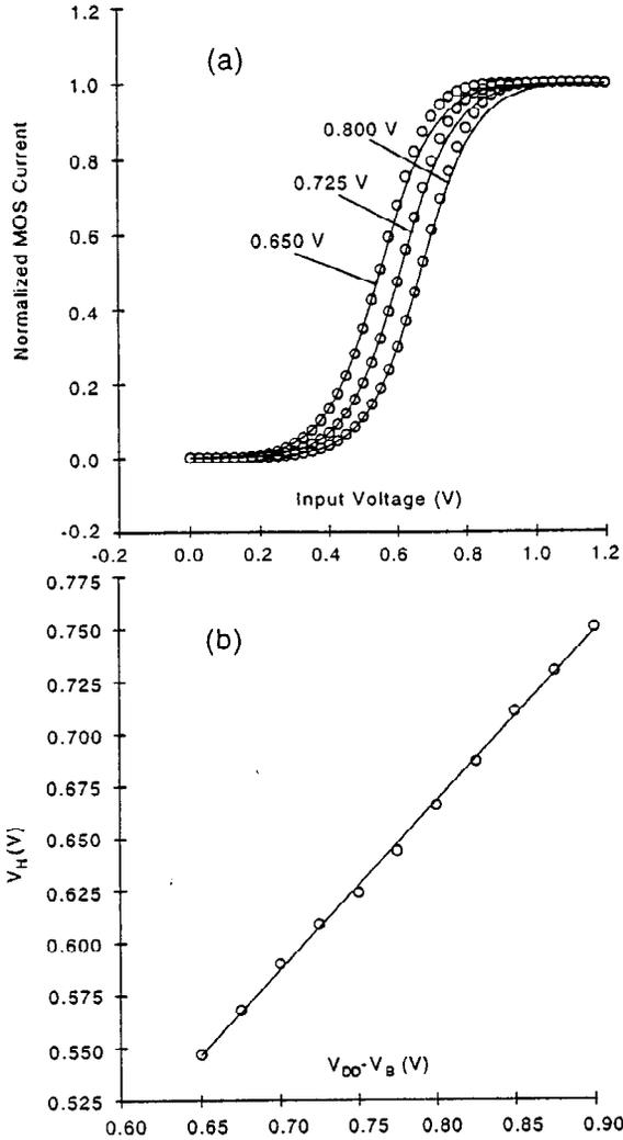
Figure A.3. The bipolar–MOS characteristics. (a) The sigmoid-like competition between the MOS and bipolar transistors as the input voltage is varied. The three parametric voltages refer to the value of the bias voltage  $V_B$  of Figure 1. (b) The threshold point of this sigmoid varies with  $V_B$ .
