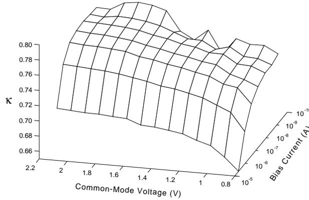
Fig. 8. The changes in  $\kappa$  in a simple  $n$ FET differential pair. The changes in  $\kappa$  are most abrupt at low common-mode voltages, i.e., at low gate-to-bulk voltages;  $\kappa$  also decreases with increasing bias current.
