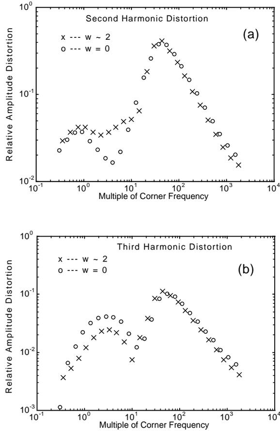
Fig. 14. Follower-integrator distortion characteristics. (a) The ratio of magnitude of the second harmonic to that of the first harmonic vs. normalized frequency, i.e., frequency normalized by the CF. (b) The same as (a) except that the third harmonic is plotted instead. Note that the addition of the  $B$  transistors decreases third harmonic distortion but increases second harmonic distortion.
