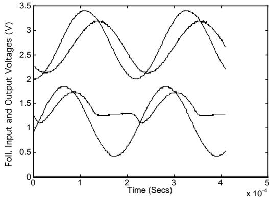
Fig. 12. Bipolar effects in the follower-integrator. The top portion of the figure shows normal follower-integrator operation, i.e., the filtering of a sinuswave input. The output waveform is attenuated and phase-shifted with respect to the input waveform. The bottom portion of the figure shows operation of the filter at low input voltages. An explanation for the strange output curve is given in Section 4, and is due to the effects of the parasitic bipolar transistors in our amplifier.
