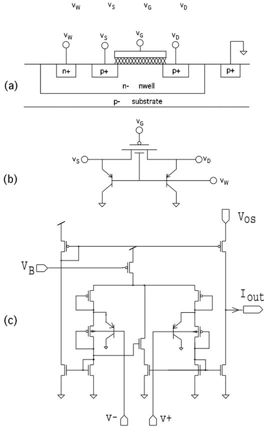
Fig. 6. The effect of the parasitic bipolar transistor. (a) A vertical cross-section of a well transistor in an  $n$ -well process. (b) The equivalent circuit of this well transistor contains two parasitic bipolar transistors. (c) The bipolar transistor at the source is responsible for shunting the amplifier's current to ground at low common-mode voltages, while the bipolar transistor at the drain plays a negligible part.
