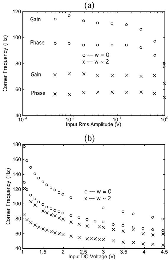
Fig. 16. Corner-frequency shifts in the follower-integrator. (a) CF-shifts vs. input rms amplitude and (b) CF-shifts vs. input dc voltage. The lower curve is the phase CF for the  $w = 0$  and the  $w = 2$  cases.
