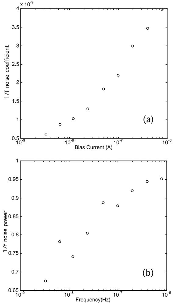
Fig. 19. Characteristics of 1/f noise. (a) The 1/f noise coefficient  $K_B$ , used in Eq. (36), as a function of the bias current  $I_B$ . (b) The 1/f noise power  $n$  as a function of the bias current  $I_B$ .
