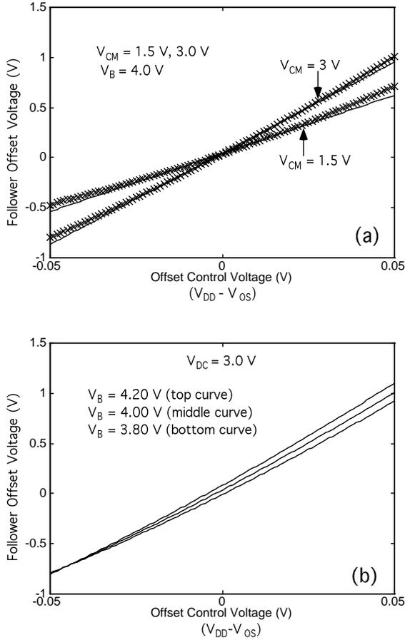
Fig. 10. Offset characteristics. (a) The offset characteristics of the amplifier at two different common-mode voltages. (b) The same characteristics at three different bias currents. More details may be found in Section 3.4.
